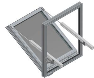
Fig.39 - mcr OSO THERM 75 smoke exhaust window with two G spindle actuators with shifted pivot point
