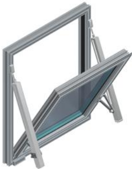
Fig.86 - mcr OSO THERM 75 smoke exhaust window with two G spindle actuators with shifted pivot point
