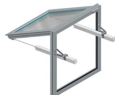
Fig. 12 - mcr OSO THERM 75 smoke exhaust window with two G spindle actuators with shifted pivot point
