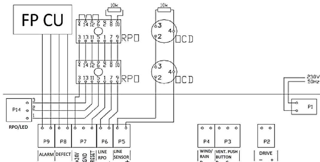
Fig. 4 Alternative connection diagram with mcr RPO-1 emergency pushbuttons and optical smoke sensors.
