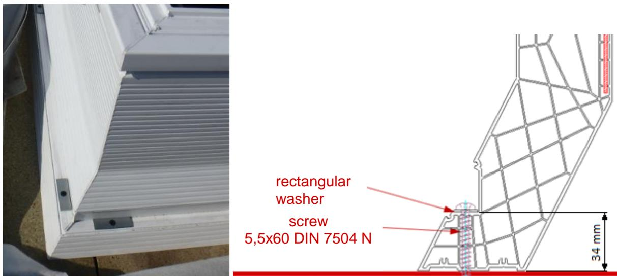
Fig. 16. Fixing the PVC base to the roof
