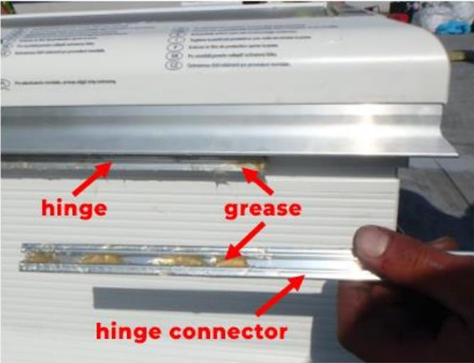
Fig. 40. Lubricating the hinge.
