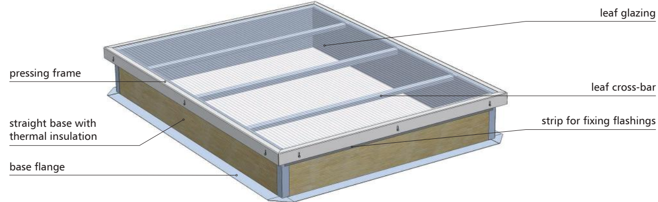
Fig.13 mcr PROLIGHT E fixed skylight design
