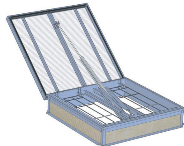
Fig.63 Safety net installed in mcr PROLIGHT C type vent
