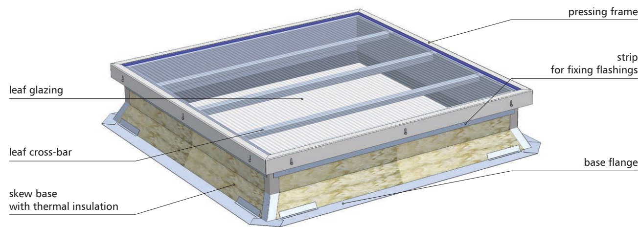
Fig.16 mcr PROLIGHT NG-A fixed skylight design
