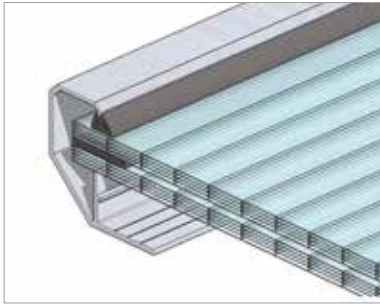
Fig.103 Skylight glazing – two multi-chamber polycarbonate panels (PCA10 + PCA10) with air gap between (PP)
