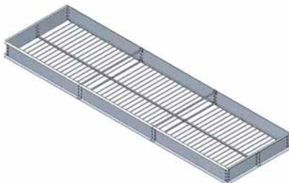
Fig.127 Anti-burglar grid installed in continuous rooflight base
