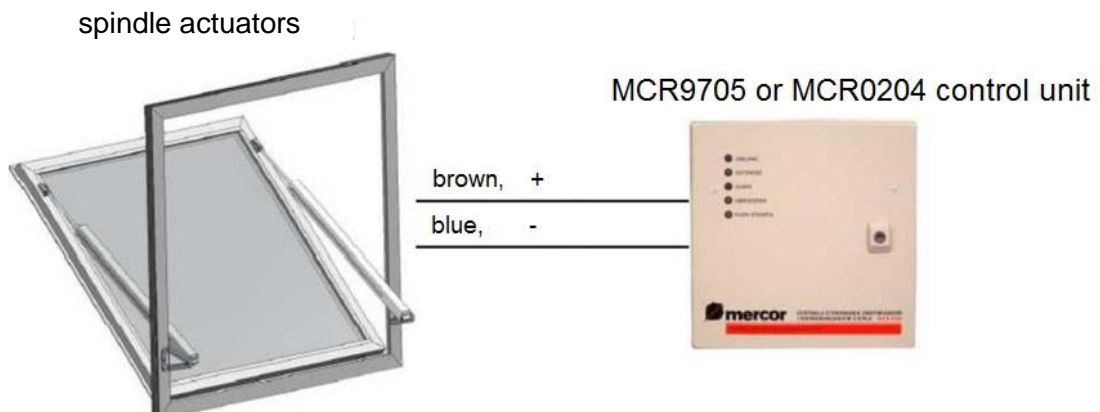
Fig. 13 Connection diagram for spindle actuators, without a lock.
