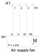
Figure 56 Fan connections circuit diagram.
