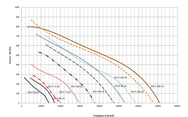
Figure 12 Parameters of standard EXi-F equipment.
