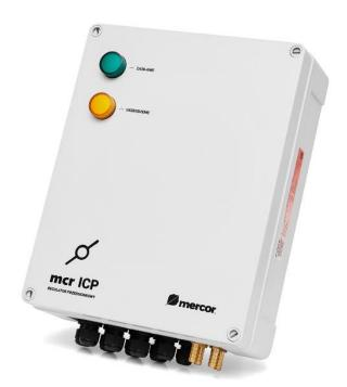
mcr ICP regulators are used where positive pressure control is required, for example in smoke-control lobbies. This maintains the target positive pressure in the protected space or the required air flow velocity through the open door opening, separating the space with increased pressure from the space without increased pressure by changing the opening rate of the control damper.
