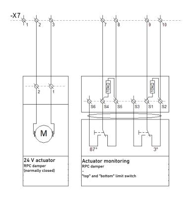
Figure 61 mcr RPC connections circuit diagram.
