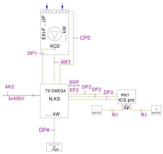
Figure 46 Schematic diagram of a vertical unit with a mcr LAM vent.
