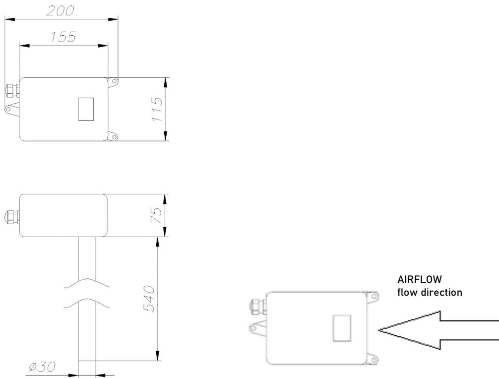
Figure 97 Installation rules along with dimensions of the SDD series sensor.
