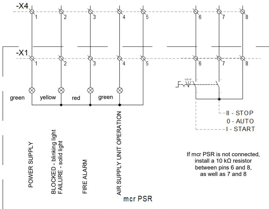
Figure 74 mcr PSR manual control panel connections circuit diagram.
