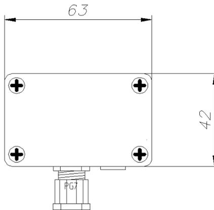
Figure 33 Overview and connection details for the MB series temperature transmitter.
