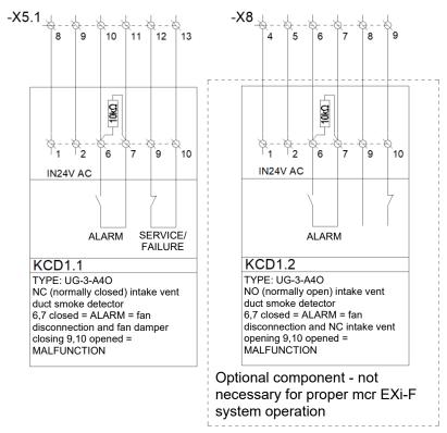
Figure 77 UG-3-A4 duct smoke detector connections circuit diagram.
