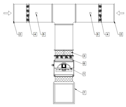
Figure 9 Sample installation of an air supply kit for the mcr EXi-F system in the roof-mounted version with a double air intake vent system: 1 - fan, 2 - intake vent, 3 - flexible connection, 4 - dampers with actuators in a double intake vent system, 5 - duct smoke detector, 6 - shut-off damper, 7 - ventilation duct.
