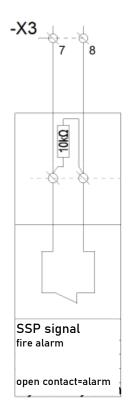
Figure 62 Connection of SSP signal (fire ALARM) to the EXi-F panel.
