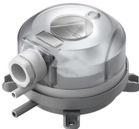
The differential pressure transmitters of the 984 series are used to measure differential pressure, overpressure and vacuum. For an optimum adaptation to the application, the transmitter can be switched between various pressure ranges. The factory setting is the most sensitive range. For the series 984M the less sensitive second range will be selected by simply removing a jumper. The output signal of the 3-wire version can be changed between 0-10 Volt and 4-20 mA by removing a jumper.
