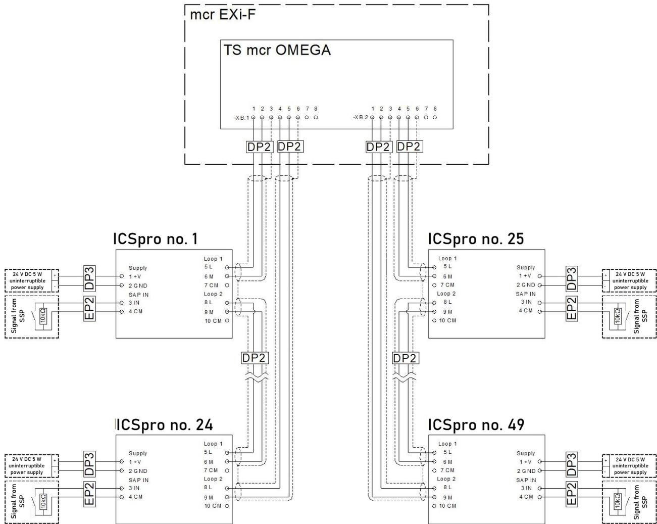
Figure 55 Block diagram for connecting mcr ICS Pro pressure transmitters in a lobby setup connected in two communication loops.
