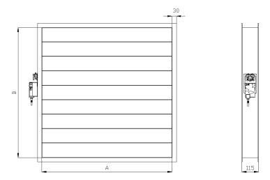
Figure 28 Overview of the EPSRC-A damper.
