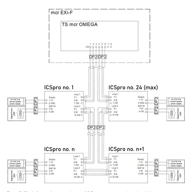
Figure 54 Block diagram for connecting mcr ICS Pro pressure transmitters in a lobby setup.
