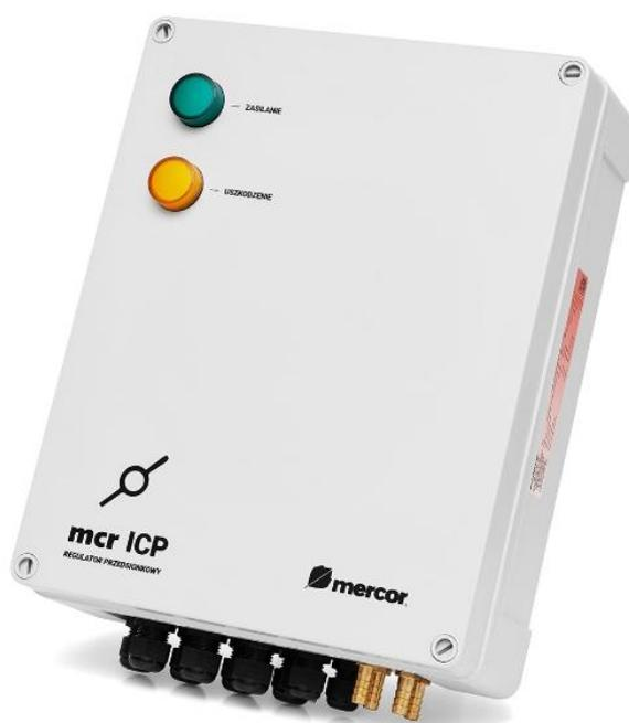
mcr ICP regulators are used where positive pressure control is required, for example in smoke-control lobbies. This maintains the target positive pressure in the protected space or the required air flow velocity through the open door opening, separating the space with increased pressure from the space without increased pressure by changing the opening rate of the control damper.
