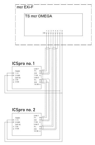
Figure 52 Block diagram for connecting mcr ICS Pro pressure transmitters in a staircase-two transmitters setup.
