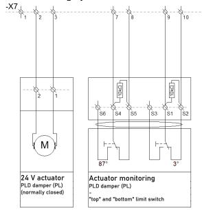
Figure 60 Connections circuit diagram for the Belimo BF, BFL, BFN series actuator.
