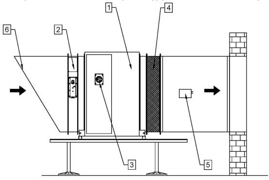
Figure 5 Sample installation of an air supply kit for the mcr EXi-F system: 1 - fan, 2 - damper with actuator, 3 - service disconnector or connection box, 4 - flexible connection, 5 duct smoke detector, 6 - inlet nozzle with grate.
