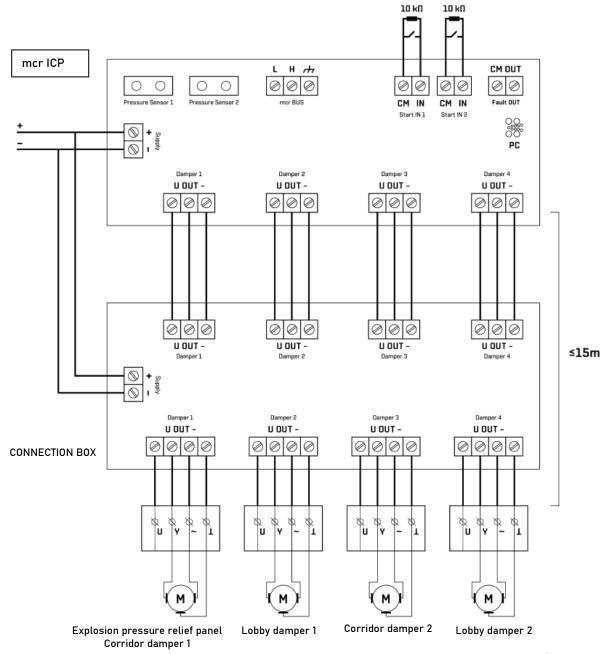
Figure 69 General block diagram for connecting mcr ICP and mcr PP regulators (support for 4 lobby dampers).
