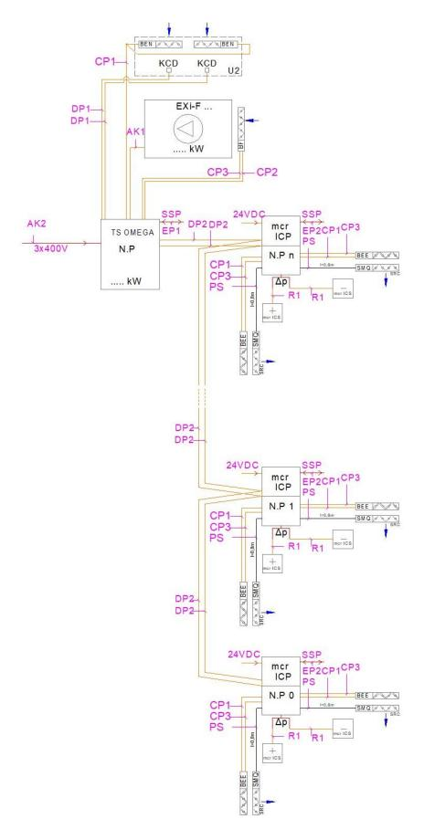
Figure 48 Schematic wiring diagram for a unit with high-speed mcr ICP dampers secured with smoke control system vents.
