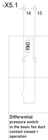
Figure 65 Pressure switch connections circuit diagram.
