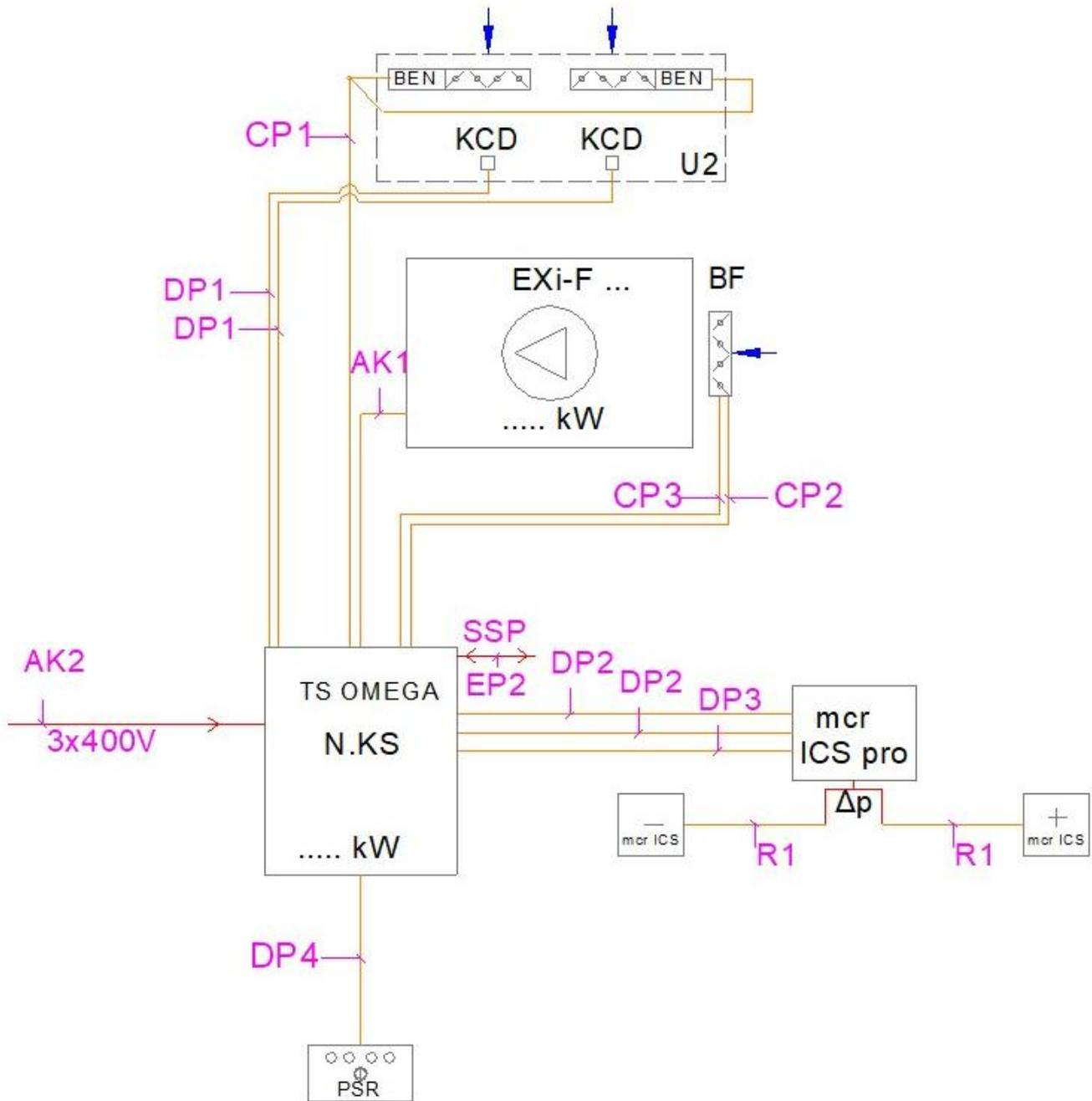
Figure 43 Schematic wiring diagram for a basic unit with a two intake vent system.
