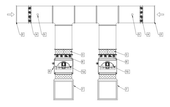
Figure 10 Sample installation of an mcr EXi-F air supply unit on the roof with a back-up unit: 1a - air supply unit basic fan, 1b - air supply unit back-up fan, 2 - intake vent, 3 - flexible connection, 4 - dampers with actuators in a double intake vent system, 5 - duct smoke detector, 6 - shut-off damper, 7 - ventilation duct, 8 - pressure switch.
