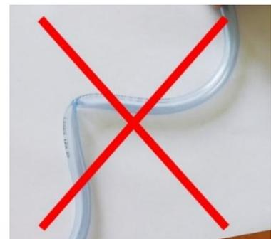
Figure 83 Principle for routing pressure hoses.
