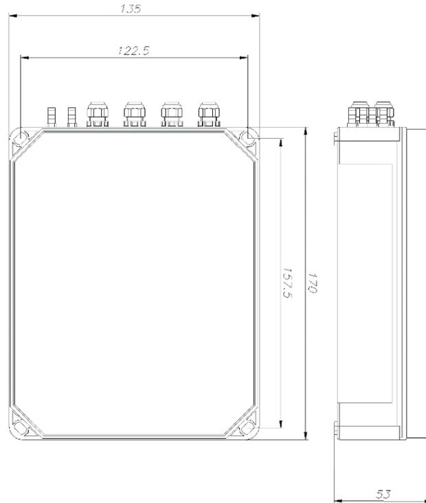
Figure 98 Dimensions of mcr ICP regulator installation holes.
