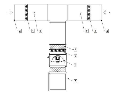
Figure 24 Sample installation of an air supply kit for the mcr EXi-F system in the roof-mounted version with two air intake vents: 1 - fan, 2 - intake vent, 3 - flexible connection, 4 - dampers with actuators in a double intake vent system, 5 - duct smoke detector, 6 - shut-off damper, 7 - ventilation duct.
