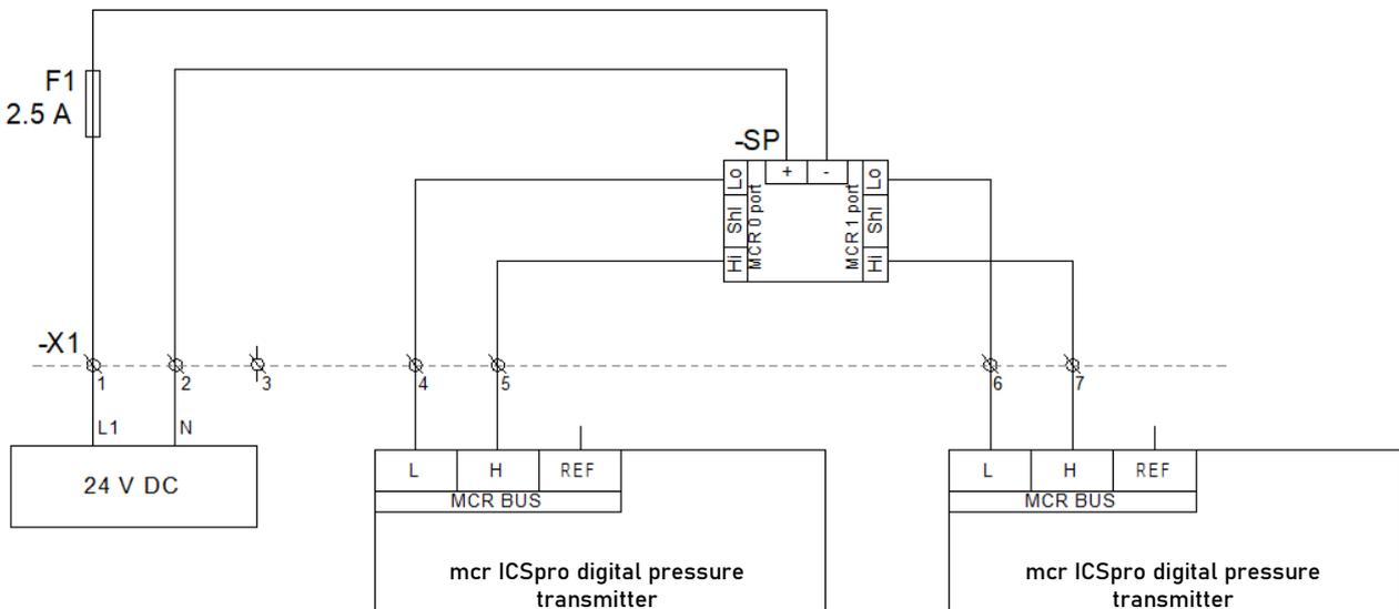
Figure 32 mcr SEP connections block diagram.
