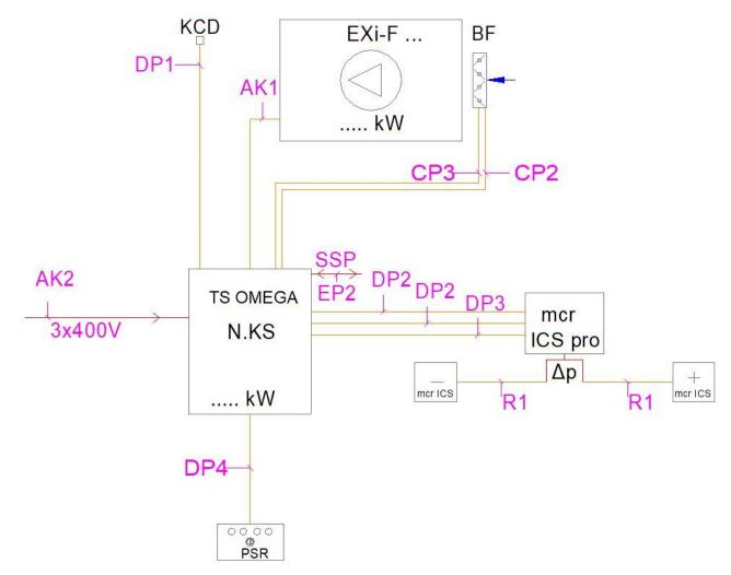
Figure 42 Schematic wiring diagram for a basic unit.
