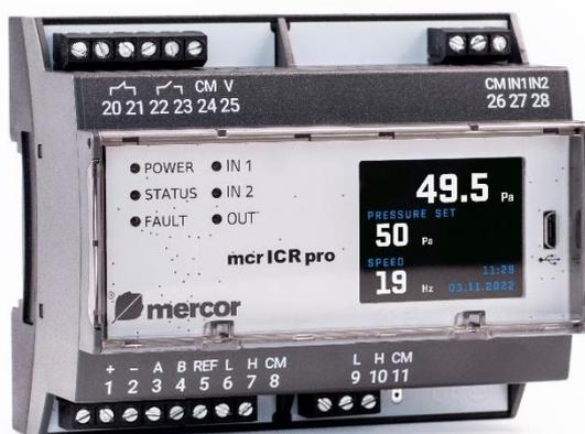
The regulator for smoke and heat control systems is an element of the mcr Omega panel that controls the rpm of the fan via a three-phase frequency converter in order to maintain the desired constant positive pressure value (20-80 Pa) in the protected zone (the device is located in the mcr Omega control panel). The measured pressure value is transferred to the regulator via a distributed network from the mcr ICR pro differential pressure sensor.
