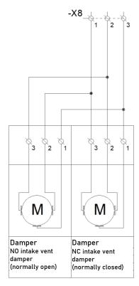
Figure 68 Connections circuit diagram for two dampers in the intake vent switching system.
