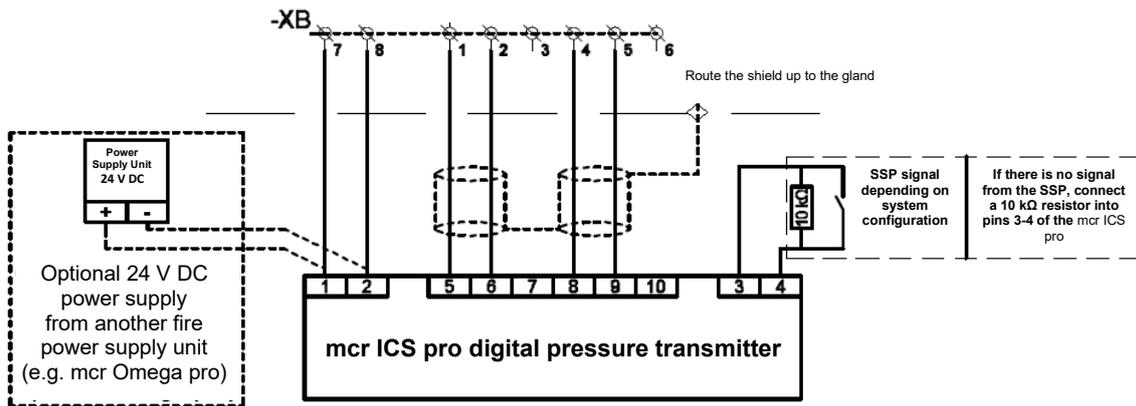
Figure 73 mcr ICS pro differential pressure transmitter connections circuit diagram
