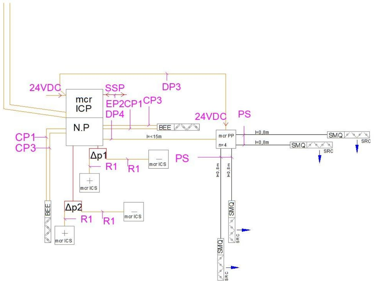
Figure 50 Schematic diagram for connecting four high-speed dampers to the mcr ICP high-speed damper regulator through a mcr PP box.
