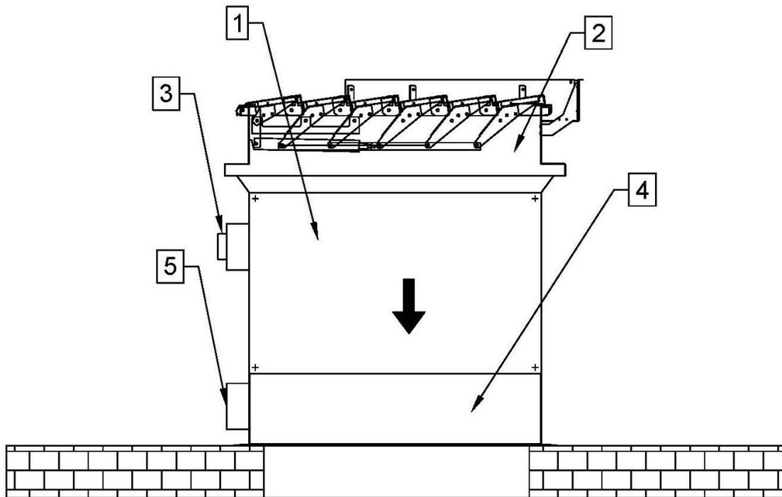
Figure 7 Sample installation of an air supply kit for the mcr EXi-F system in the UP version on the roof: 1 - fan, 2 - LAM vent with actuator, 3 - service disconnect or connection box, 4 - roof base, 5 - duct smoke detector.
