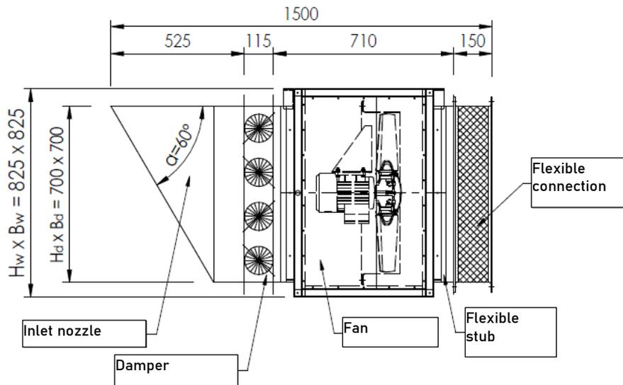
Figure 89 Basic dimensions of the standard mcr EXi-F 63-1 air supply units in a box-type housing - horizontal installation.
