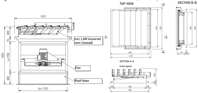
Figure 94 Vertical installation with louvered vent: mcr EXi-F 90-1S UP,90-2S UP,100-1S UP,100-2 S UP.
