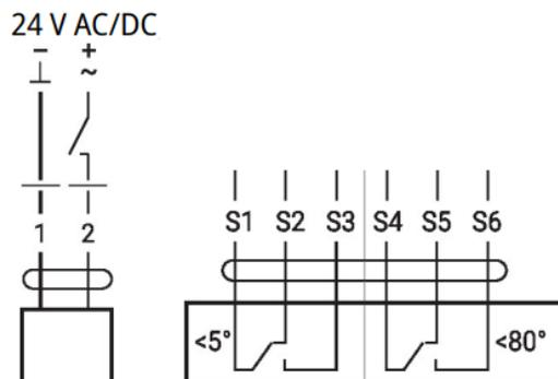
Figure 80 Connections circuit diagram for the Belimo BF/BFL/BFN series actuator. Actuators used in shut-off dampers at mcr EXi-F air supply units.
