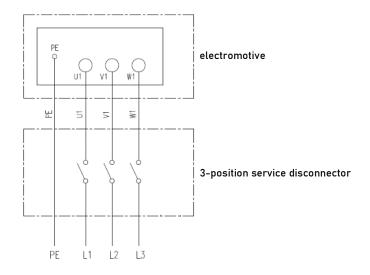
Figure 58 Electrical diagram of the service disconnector for the air supply unit fan.
