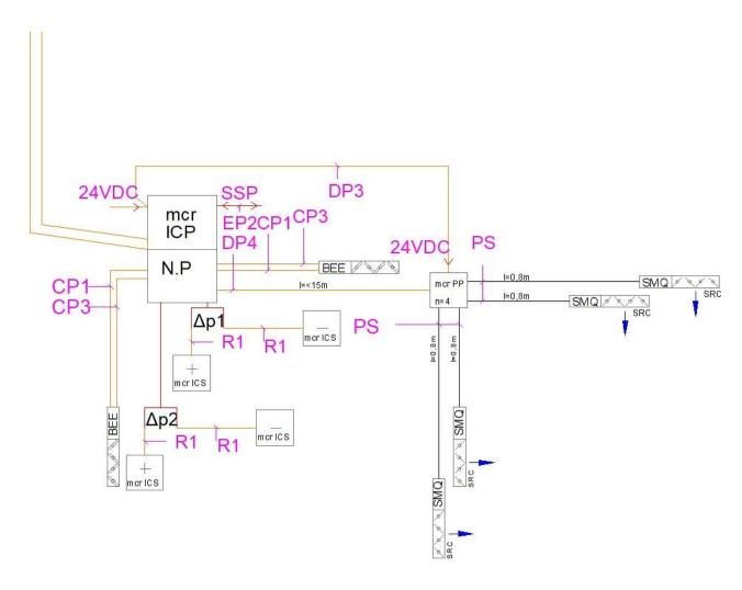
Figure 50 Schematic diagram for connecting four high-speed dampers to the mcr ICP high-speed damper regulator thorough a mcr PP box.
