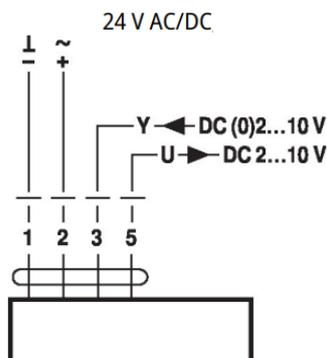
Figure 82 Connections circuit diagram for the Belimo NMQ/LMQ/SMQ series actuator.
