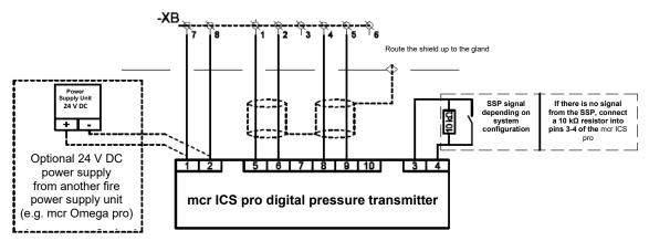
Figure 73 mcr ICS pro differential pressure transmitter connections circuit diagram
