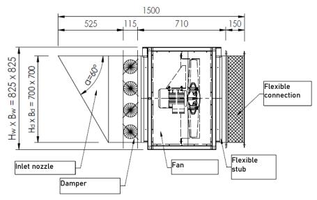
Figure 89 Basic dimensions of the standard mcr EXi-F 63-1 air supply units in a box-type housing - horizontal installation.
