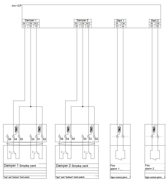
Figure 72 Connection diagram for fire ventilation vent limit switches and SSP alarms.
