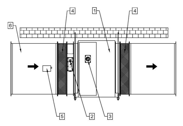
Figure 6 Sample installation of an air supply kit for the mcr EXi-F system in the duct version: 1 - fan, 2 - damper with actuator, 3 - service disconnector or connection box, 4 - flexible connection, 5 duct smoke detector.
