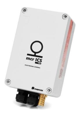
The device is used to measure the differential pressure in a space protected by increased pressure (staircases, elevator shafts or smoke-control lobbies). Two pressure lines should be connected to the device. The measurement results are transferred in real-time through the digital interface of the regulator that controls fan operation (via the inverter).
