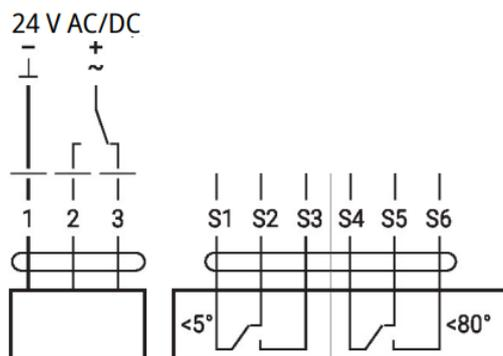
Figure 81 Connections circuit diagram for the Belimo BE/BEE/BLE series actuator. Actuators used in dampers in double intake vent systems.
