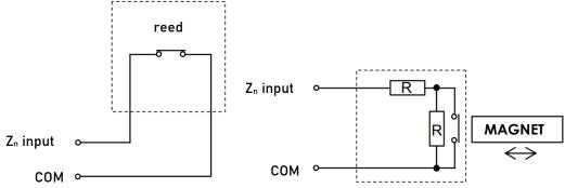
Figure 35 Manners of connecting magnetic sensors (reeds).
