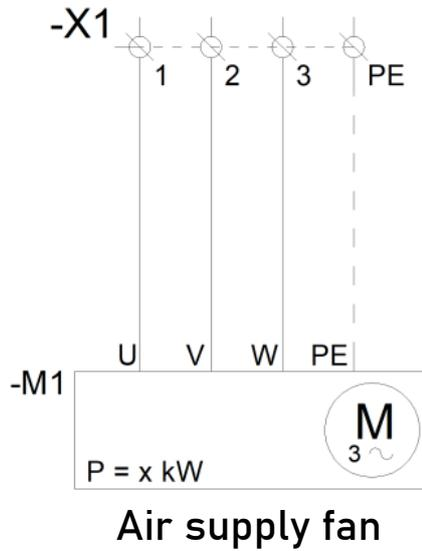
Figure 66 Fan connections circuit diagram
