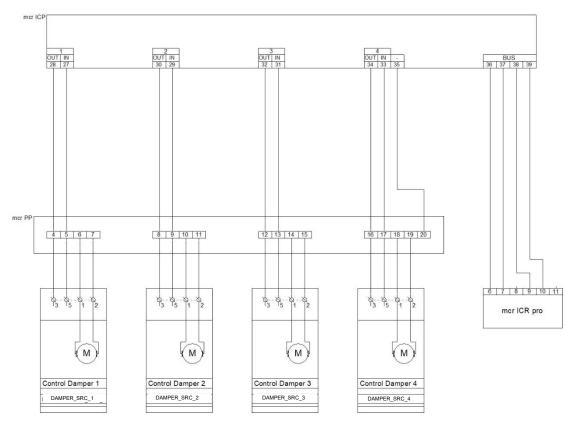
Figure 70 Block diagram for connecting a mcr ICP regulator in the communications network with mcr Omega.
