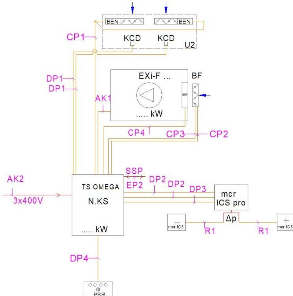
Figure 45 Schematic wiring diagram for a unit with a double intake vent system and mcr HT anti-icing system.
