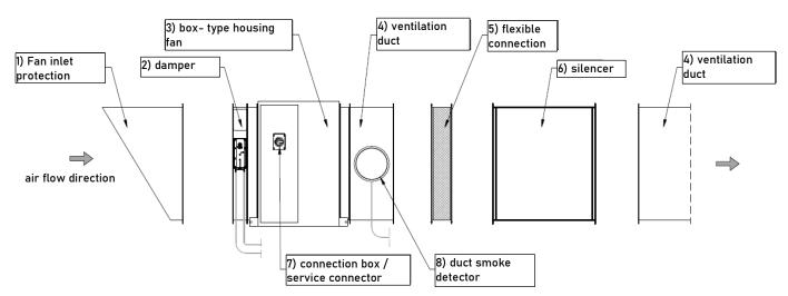
Figure 88 Sample standard horizontal installation of a set of mcr EXi-F system components: 1 - fan inlet protection, 2 - damper, 3 - mcr Monsun E1 fan in a box-type housing 4 - ventilation duct (pipe), 5 - flexible connection, 6 - silencer, 7 - connection box / service connector, 8 - duct smoke detector.
