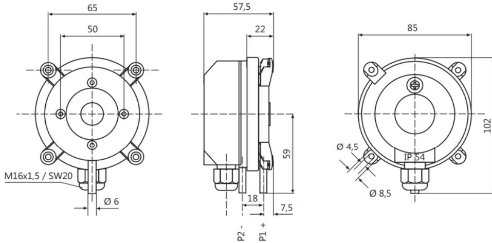
Figure 36 Differential pressure switch overview.
