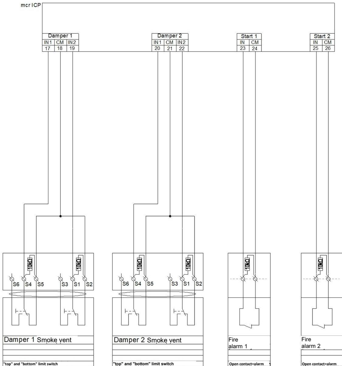
Figure 72 Connection diagram for fire ventilation vent limit switches and SSP alarms.
