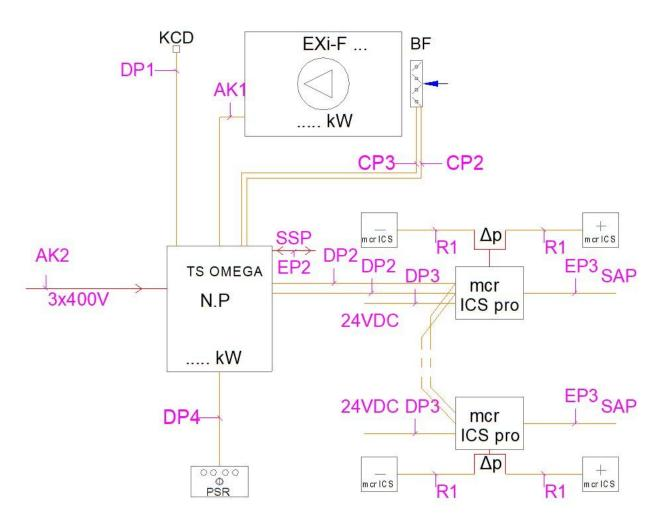
Figure 47 Schematic wiring diagram for lobby air supply.
