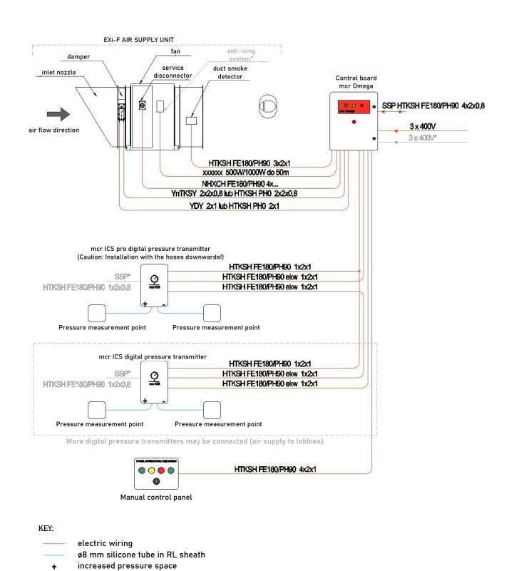
Figure 40 Wiring of the basic EXi-F unit.
