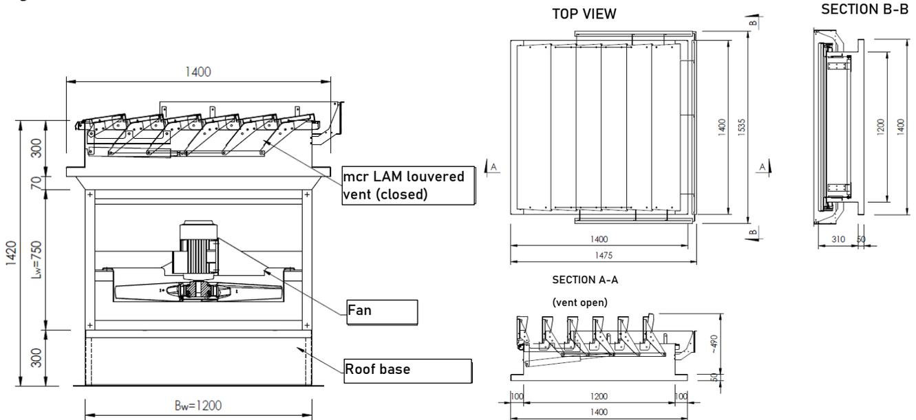
Figure 94 Vertical installation with louvered vent: mcr EXi-F 90-1S UP,90-2S UP,100-1S UP,100-2 S UP.
