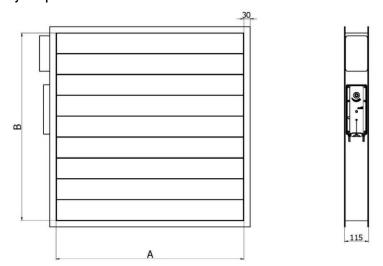
Figure 13 Overview of a shut-off damper.
