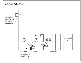
Figure 2 Design requirements diagram for solutions A and B.
