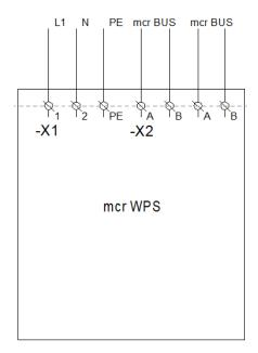
Figure 76 Electrical connection of the mcr WPS panel (U=230 V AC).
