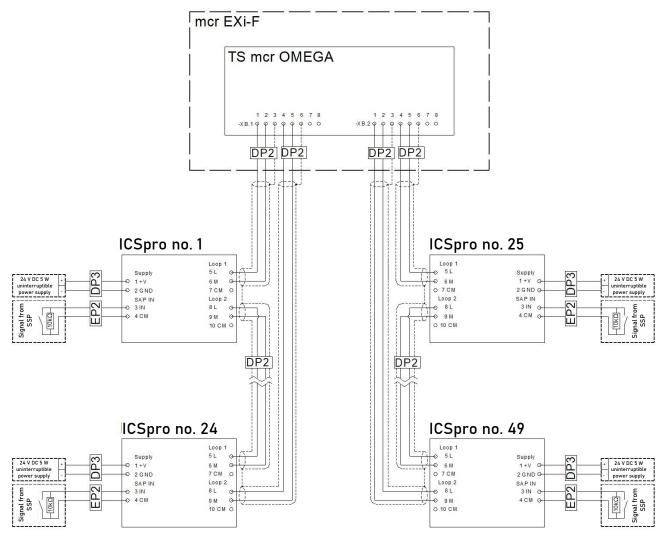
Figure 55 Block diagram for connecting mcr ICS Pro pressure transmitters in a lobby setup connected in two communication loops.
