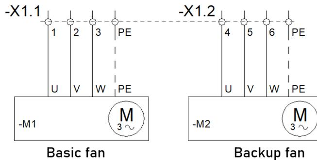
Figure 64 Fans connections circuit diagram.
