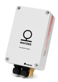
The device is used to measure the differential pressure in a space protected by increased pressure (staircases, elevator shafts or smoke-control lobbies). Two pressure lines should be connected to the device. The measurement results are transferred in real-time through the digital interface of the regulator that controls fan operation (via the inverter) or may be autonomic regulator. It can be change in device menu.
