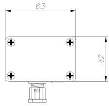
Figure 33 Overview and connection details for the MB series temperature transmitter.
