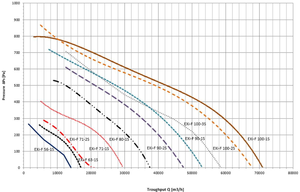
Figure 12 Parameters of standard EXi-F equipment.
