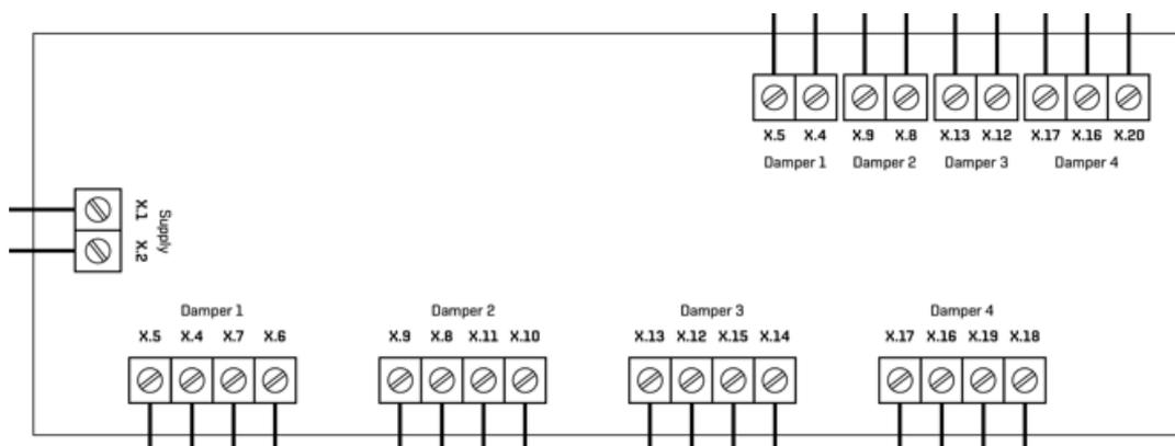
Figure 27 Terminals in the mcr PP box.
