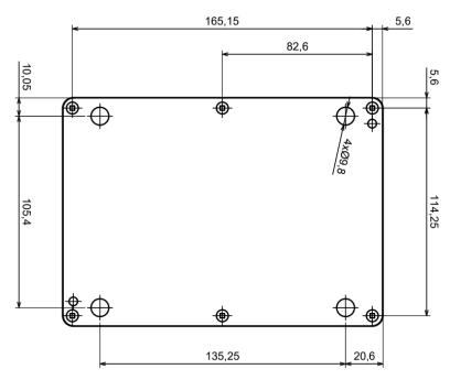
Figure 96 Dimensions of available mcr PSR/PRSC installation holes.
