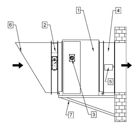
Figure 8 Sample installation of an air supply kit for the mcr EXi-F system in the wall-mounted version indoors: 1 - fan in a box-type housing, 2 - damper with actuator, 3 - service disconnector or connection box, 4 - lead, 5 - duct smoke detector, 6 - inlet nozzle with grate, 7 - supporting structure.
