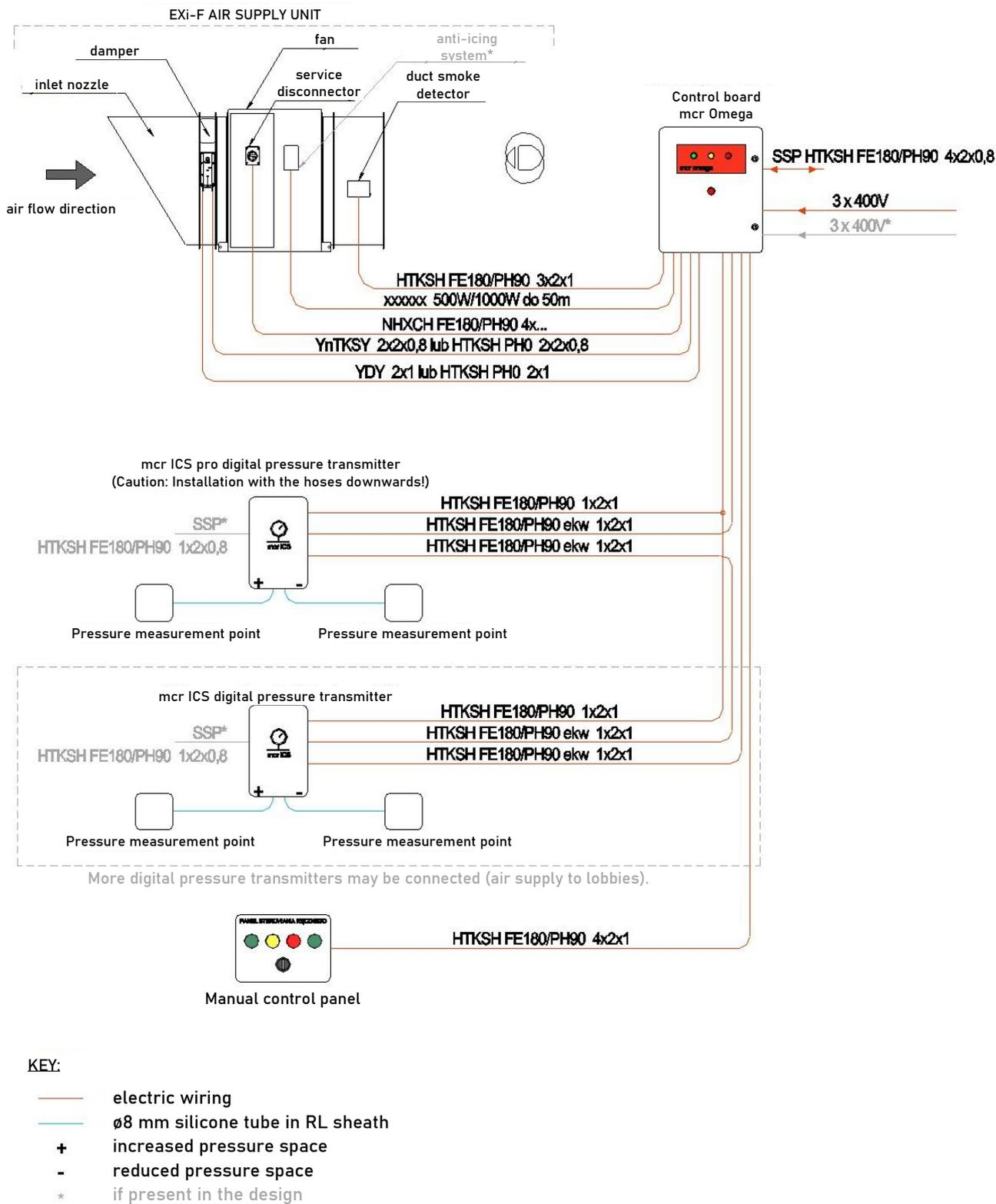
Figure 40 Wiring of the basic EXi-F unit.
