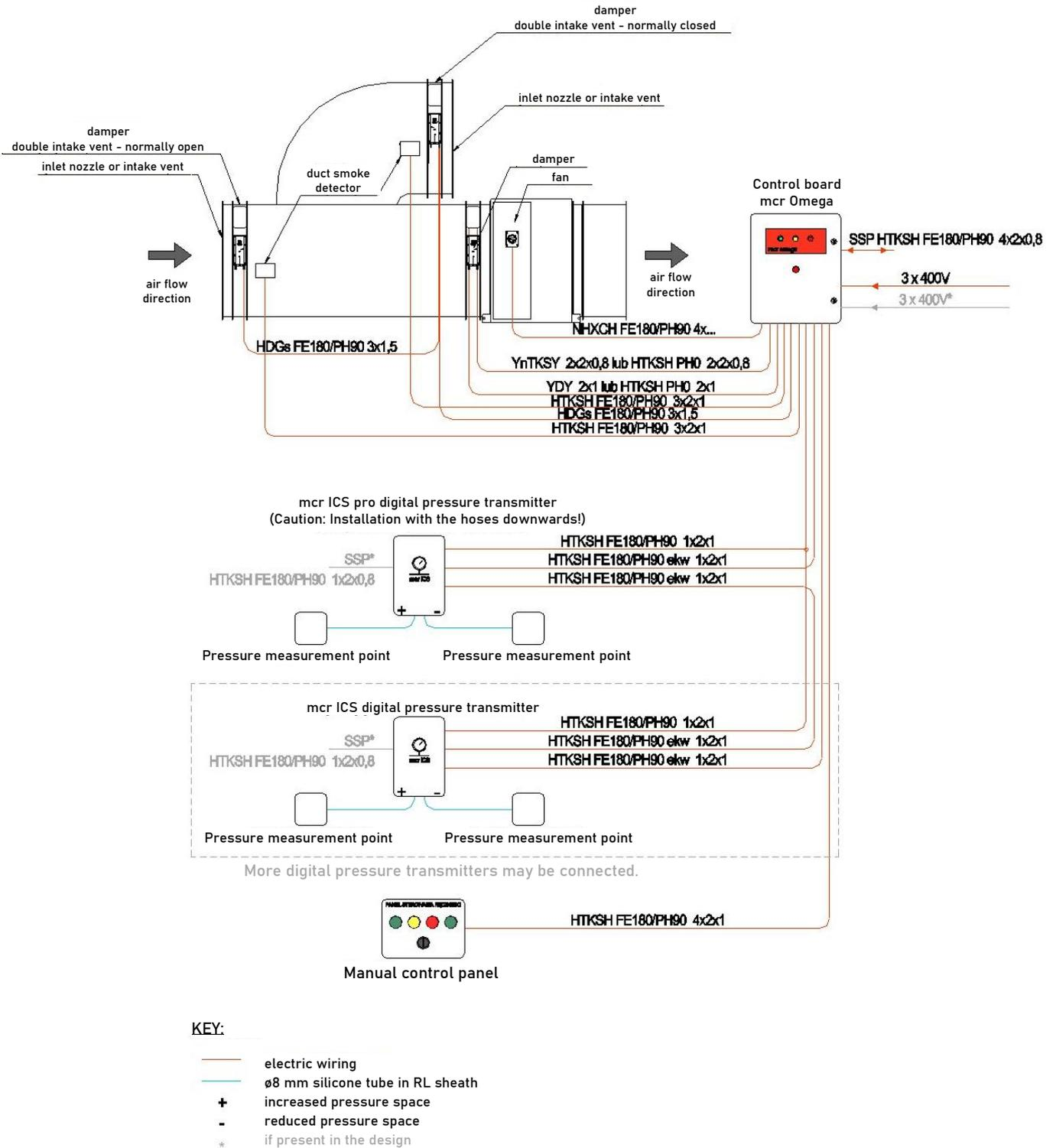
Figure 41 Wiring of the EXi-F unit with a two intake vent system.
