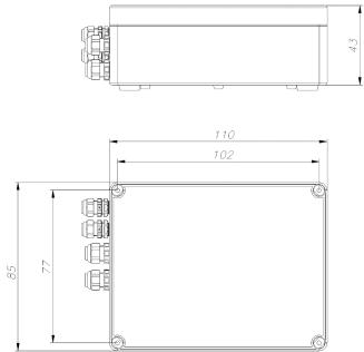
Figure 100 Dimensions of mcr SEP network separator installation holes.
