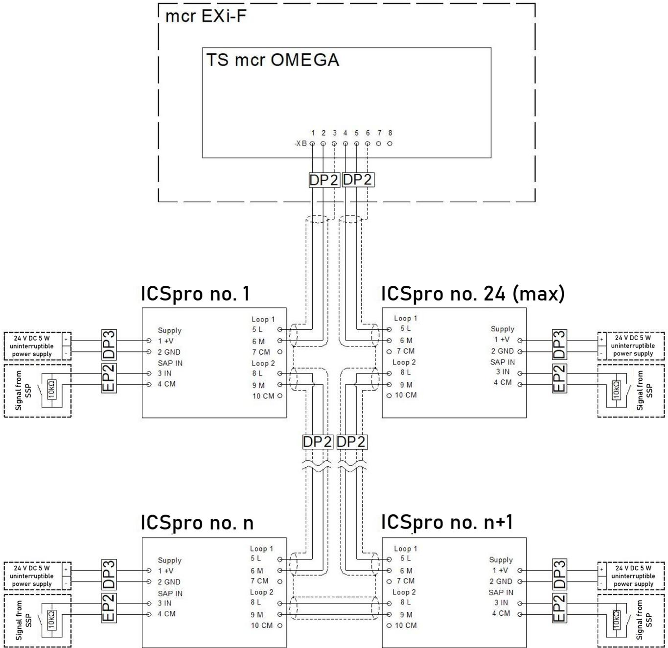
Figure 54 Block diagram for connecting mcr ICS Pro pressure transmitters in a lobby setup.
