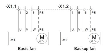
Figure 64 Fans connections circuit diagram.
