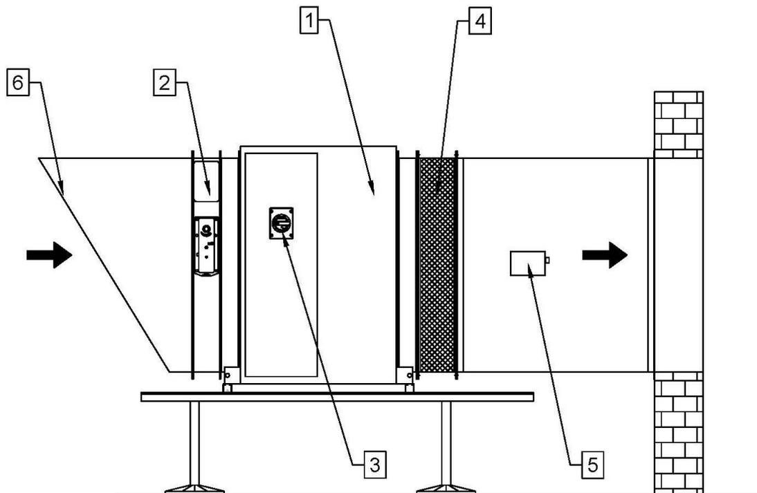
Figure 5 Sample installation of an air supply kit for the mcr EXi-F system: 1 - fan, 2 - damper with actuator, 3 - service disconnect or connection box, 4 - flexible connection, 5 duct smoke detector, 6 - inlet nozzle with grate.
