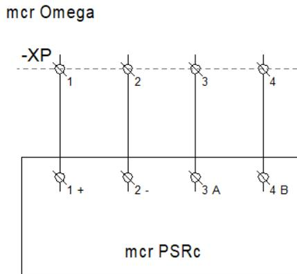
Figure 75 mcr PSRC manual control panel connections circuit diagram.
