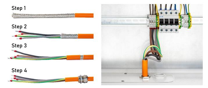
Figure 57 Step by step wire preparation guide.
