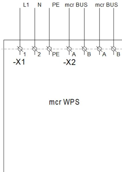
Figure 76 Electrical connection of the mcr WPS panel (U=230 V AC).
