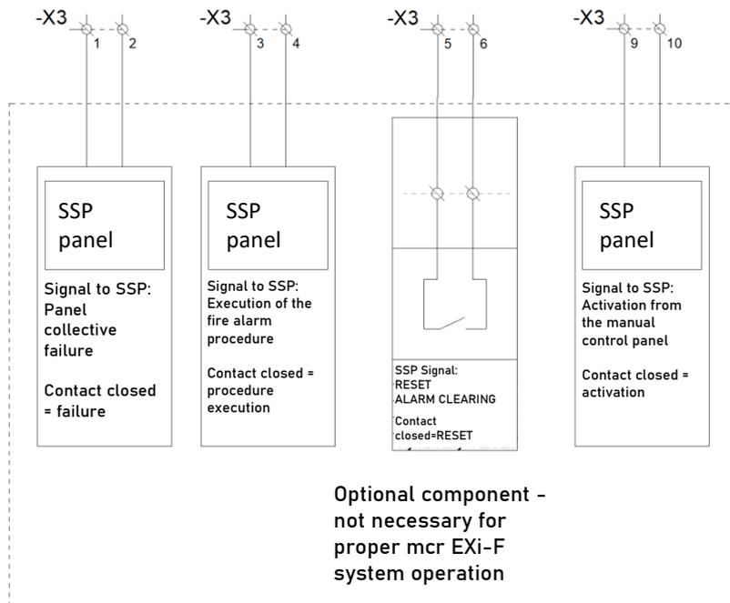
Figure 63 Connecting optional SSP signals to the mcr Omega panel.
