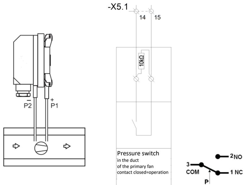
Figure 37 Electrical diagram of a LF or DW series differential pressure switch.
