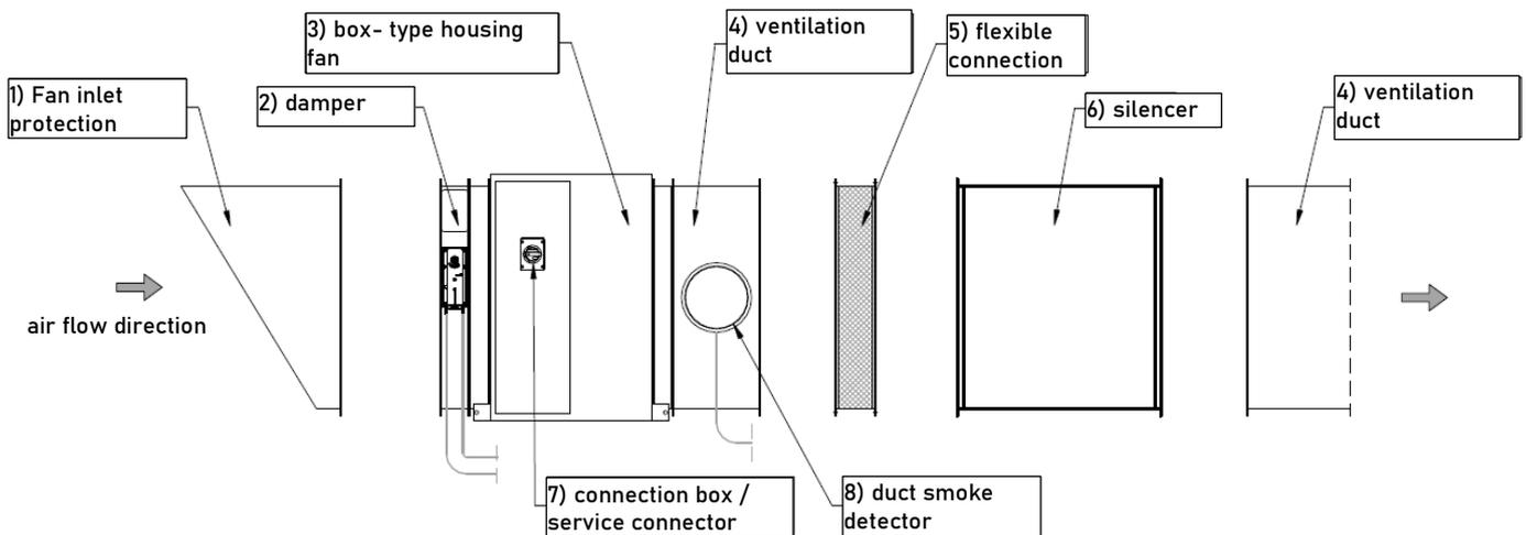
Figure 88 Sample standard horizontal installation of a set of mcr EXi-F system components: 1 - fan inlet protection, 2 - damper, 3 - mcr Monsun E1 fan in a box-type housing 4 - ventilation duct (pipe), 5 - flexible connection, 6 - silencer, 7 - connection box / service connector, 8 - duct smoke detector.
