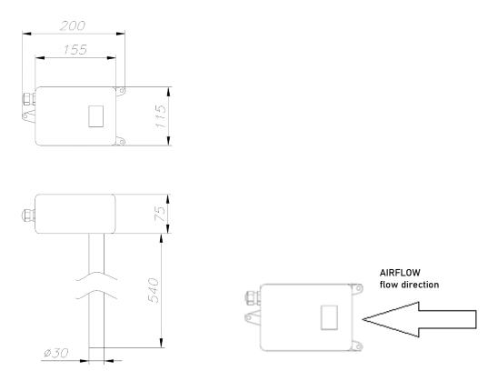
Figure 97 Installation rules along with dimensions of the SDD series sensor.
