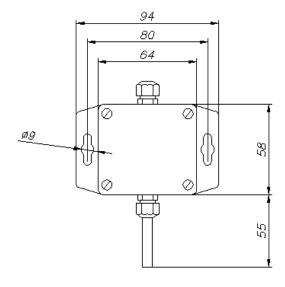
Figure 34 Overview for the AR series temperature transmitter.
