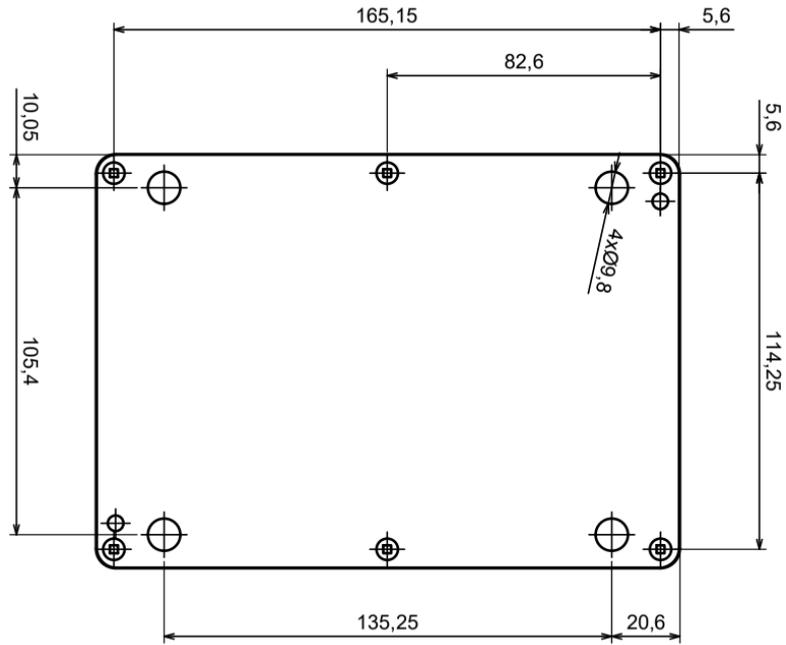
Figure 96 Dimensions of available mcr PSR/PRSC installation holes.
