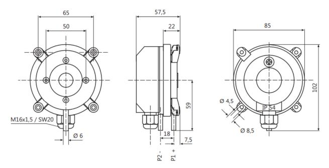
Pressure input P1 (+) is connected downstream from the fan. Pressure input P2 (-) is connected upstream from the fan.
