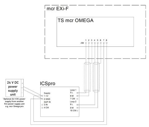
Figure 51 Block diagram for connecting a mcr ICS Pro pressure transmitter in a staircase-single transmitter setup.
