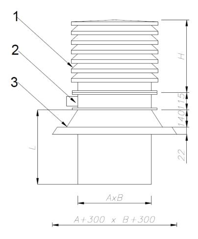
Figure 21 Detailed view of the RPC protected space unsealing module. 1. exhaust vent, 2 damper with BFN actuator, 3 roof base.
