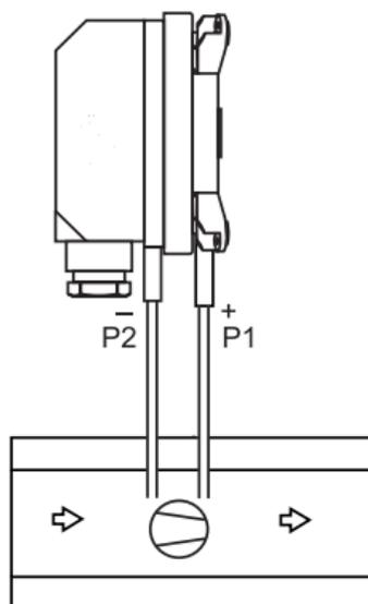
*Figure 103 Installation diagram of a LF series differential pressure switch.*
