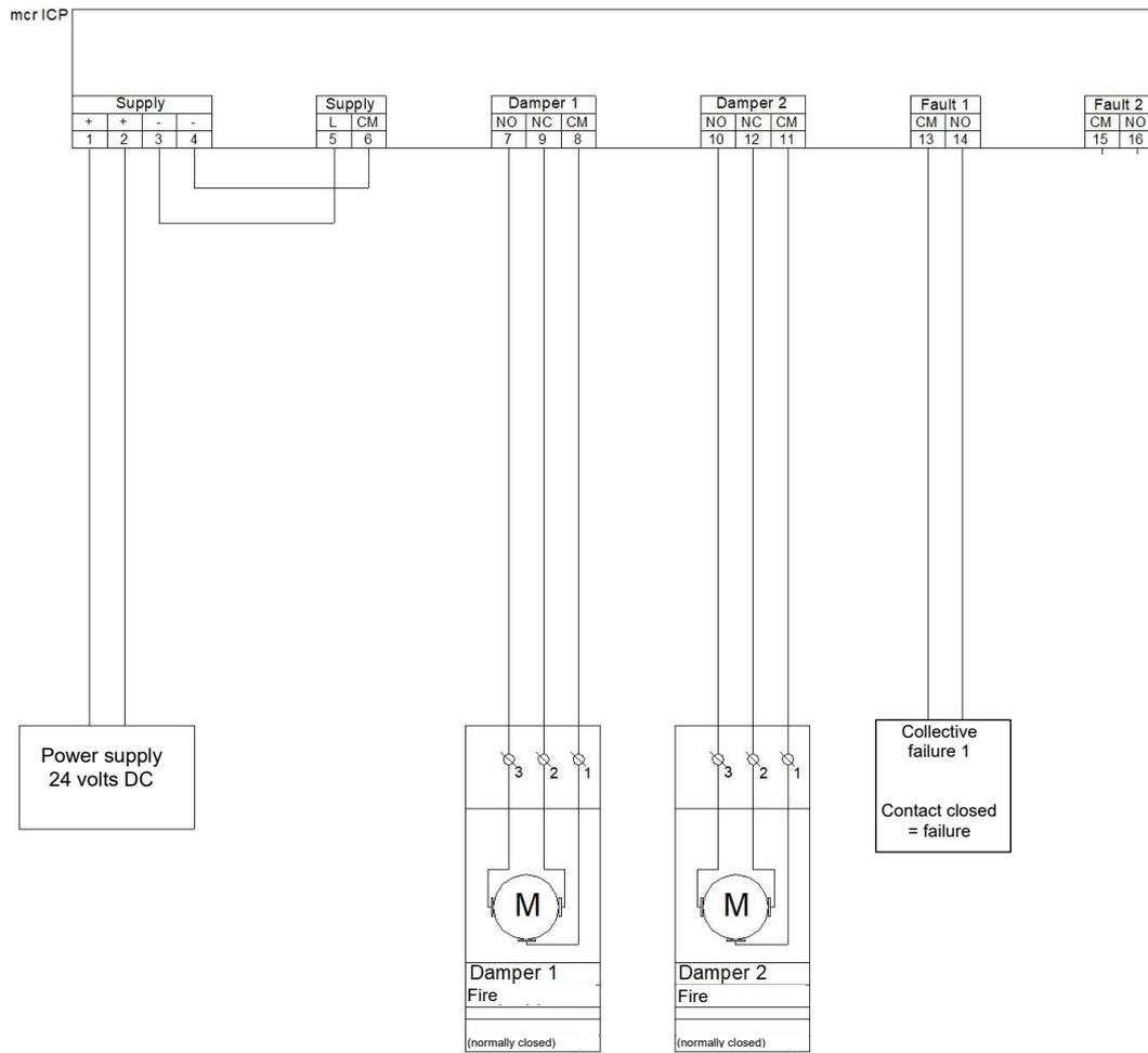
Figure 71 Block diagram for connecting a mcr ICP regulator – option with support for fire ventilation vents.
