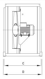
Figure 11 Installation dimensions of mcr EXi-F system air supply unit fans.
