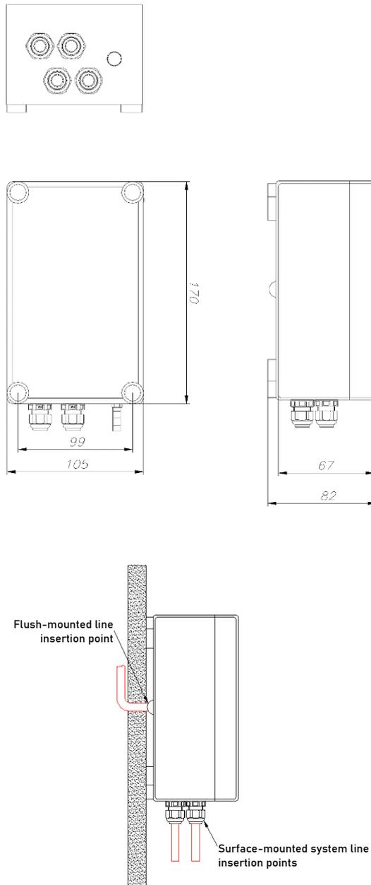
Figure 95 ICS pro transmitter installation dimensions.
