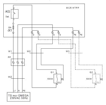
Figure 30 Internal HT system connections circuit diagram.
