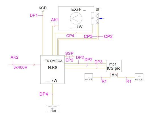
Figure 44 Schematic wiring diagram for a unit with the mcr HT anti-icing system.
