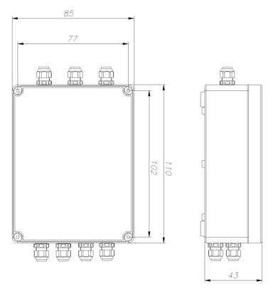
Figure 99 Dimensions of mcr PP connection box installation holes.
