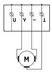
Figure 25 Connections circuit diagram for the Belimo NMQ/LMQ/SMQ series actuator.
