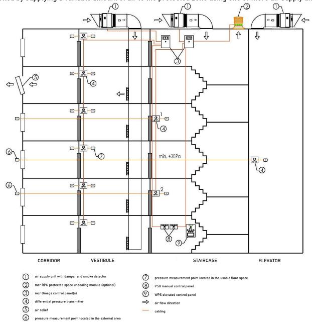
Figure 1 mcr EXi-F system schematic diagram.
