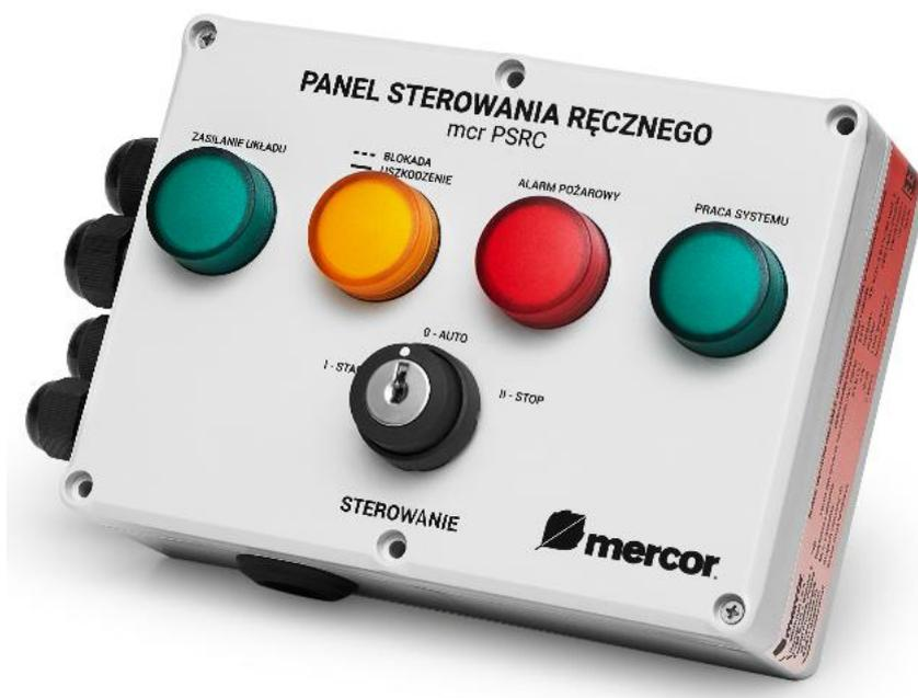
An elevated manual control panel is used to control the system from a distance using a key switch. It allows the lead firefighter to manually activate or deactivate the pressurization smoke control system. The panel should be placed near emergency exits in areas easily accessible for emergency responders. The panel signals control panel operation and provides information about the following states:
