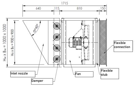
Figure 90 Basic dimensions of the standard mcr EXi-F 80-1S, 71-1S, 71-2S air supply units in a box-type housing - horizontal installation.
