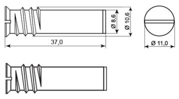
Figure 102 Installation dimensions of MC-240 series sensors.
