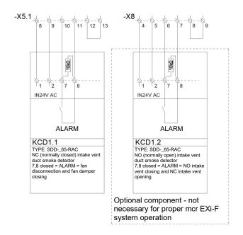
Figure 78 SDD-65-RAC duct smoke detector connections circuit diagram.
