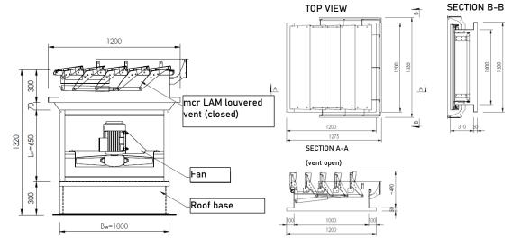
Figure 93 Vertical installation with louvered vent: mcr EXi-F 71-1S UP, 71-2S UP, 80-1S UP.
