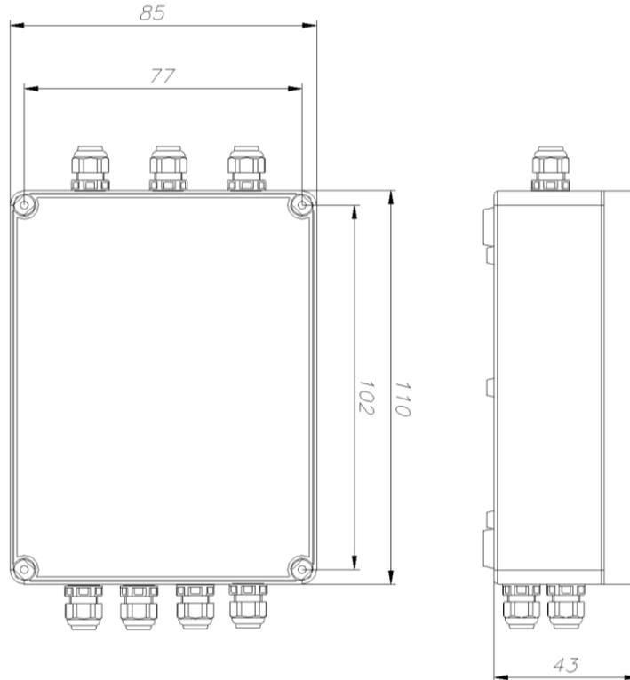
Figure 99 Dimensions of mcr PP connection box installation holes.
