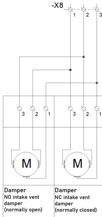
Figure 68 Connections circuit diagram for two dampers in the intake vent switching system.
