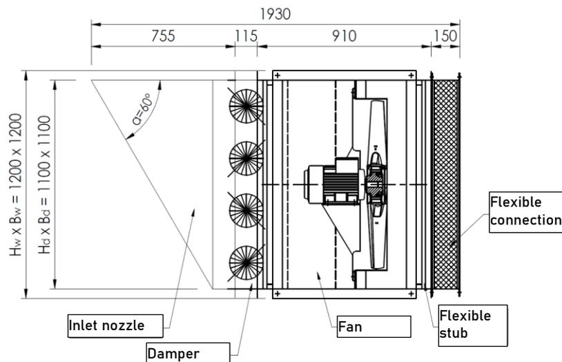
Figure 91 Basic dimensions of the standard mcr EXi-F 90-1S, 90-2S, 100-1S, 100-2S air supply units in a box-type housing - horizontal installation.
