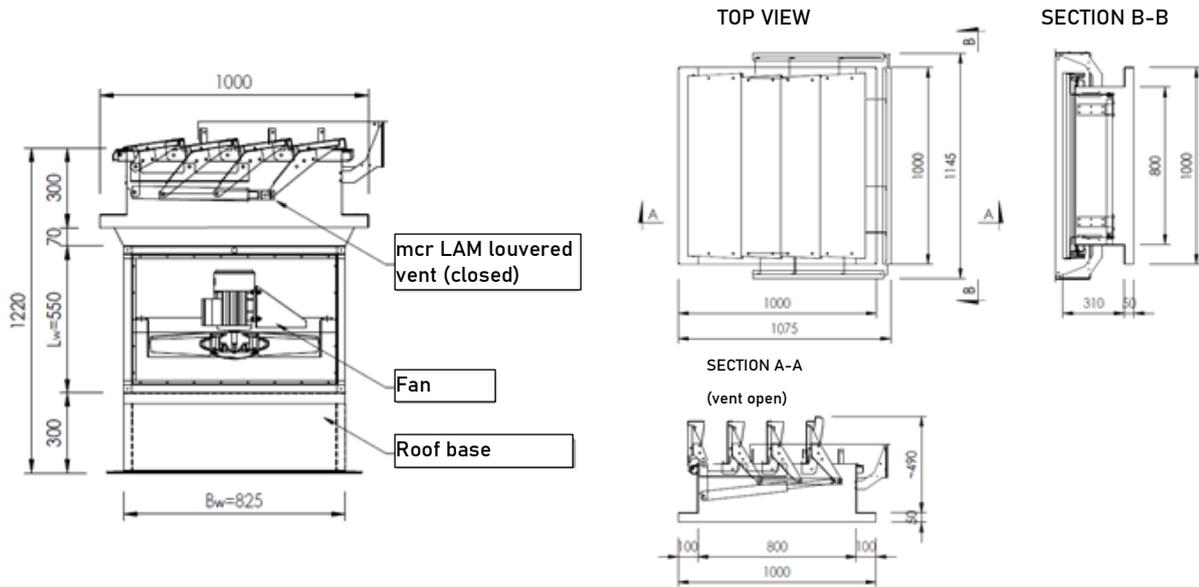
Figure 92 Vertical installation with louvered vent: mcr EXi-F 63- 1S UP.
