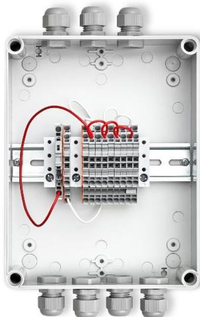
Connecting actuators to the controller can be done through a dedicated connection box. The box is equipped with a thermal fuse. The total length of cables between the controller and the actuator must not exceed 15 m. External box dimensions: 220x170x86mm.
