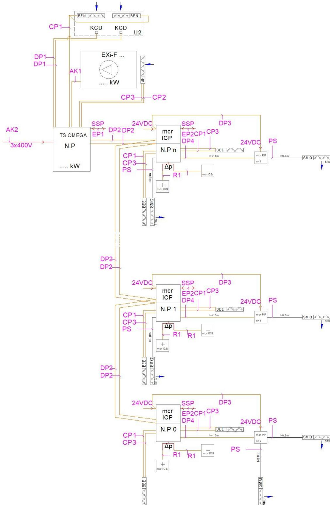
Figure 49 Schematic wiring diagram for a unit with high-speed mcr ICP dampers secured with smoke control system vents located at a higher distance from the regulator, using an mcr PP box.
