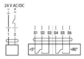
Figure 80 Connections circuit diagram for the Belimo BF/BFL/BFN series actuator. Actuators used in shut-off dampers at mcr EXI-F air supply units.
