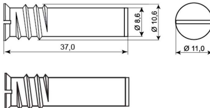
Figure 102 Installation dimensions of MC-240 series sensors.
