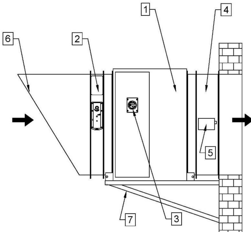
Figure 8 Sample installation of an air supply kit for the mcr EXi-F system in the wall-mounted version indoors: 1 - fan in a box-type housing, 2 - damper with actuator, 3 - service disconnect or connection box, 4 - lead, 5 - duct smoke detector, 6 - inlet nozzle with grate, 7 - supporting structure.
