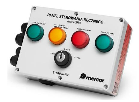
An elevated manual control panel is used to control the system from a distance using a key switch. It allows the lead firefighter to manually activate or deactivate the pressurization smoke control system. The panel should be placed near emergency exits in areas easily accessible for emergency responders.
