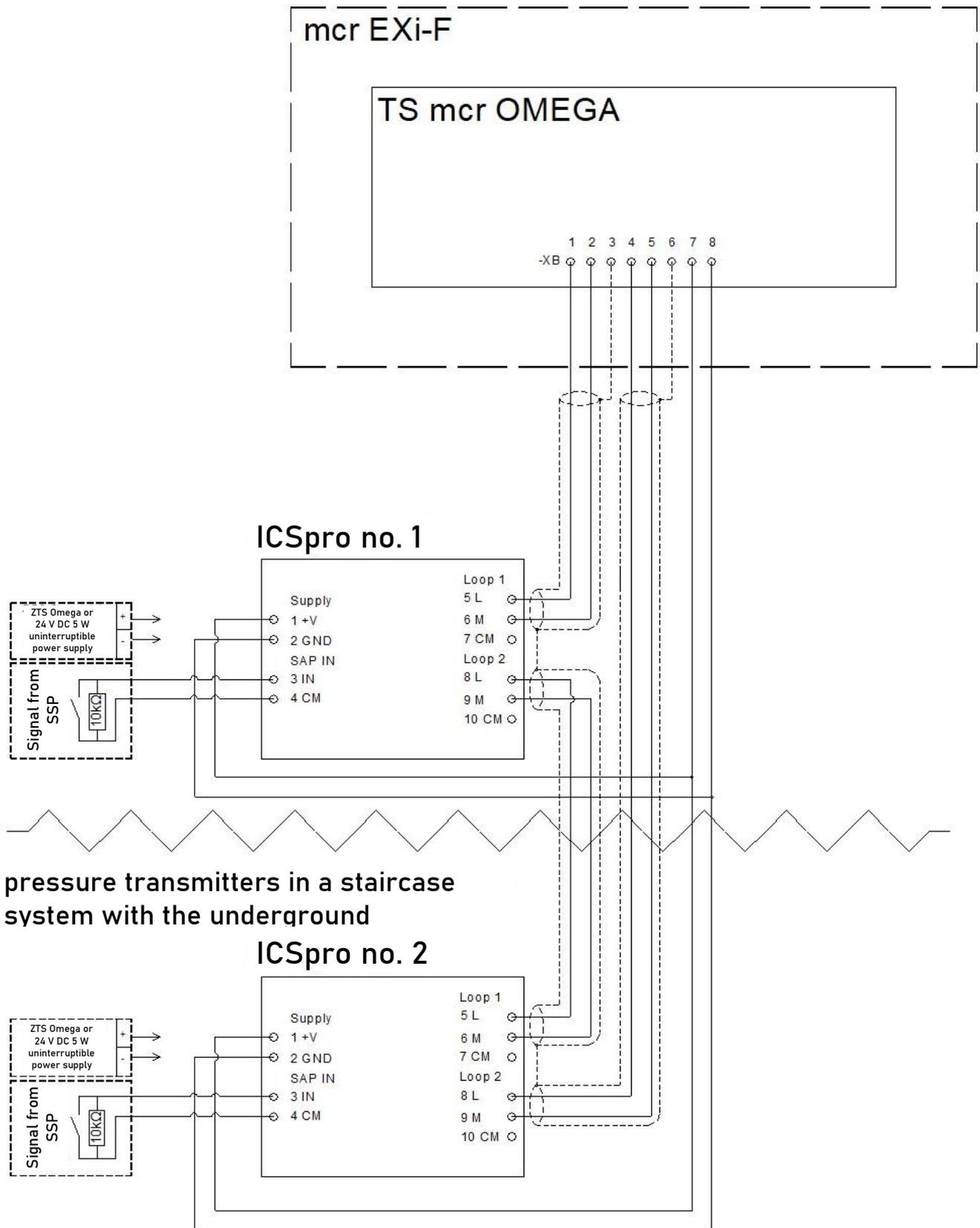
Figure 53 Block diagram for connecting mcr ICS Pro pressure transmitters in a staircase system with separate transmitters in the underground part triggered from the FSS.
