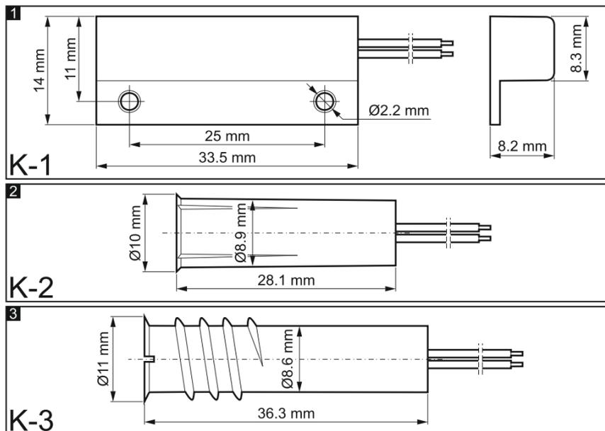
Figure 101 K-x series sensor installation dimensions.
