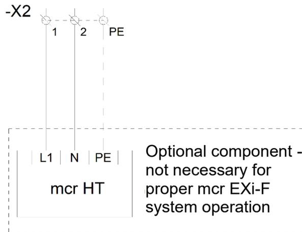
Figure 79 Electrical connection of the mcr Omega panel for the anti-icing system.
