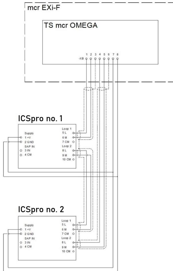
Figure 52 Block diagram for connecting mcr ICS Pro pressure transmitters in a staircase-two transmitters setup.
