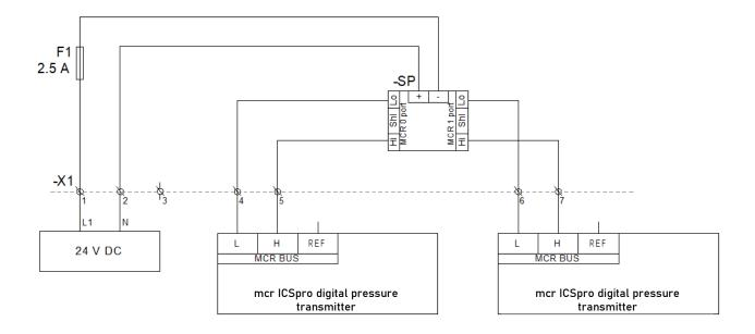
Figure 32 mcr SEP connections block diagram.
