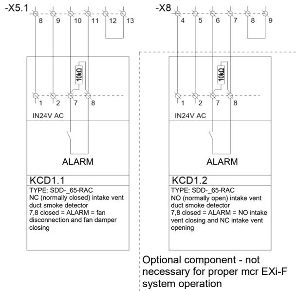
Figure 78 SDD-65-RAC duct smoke detector connections circuit diagram.
