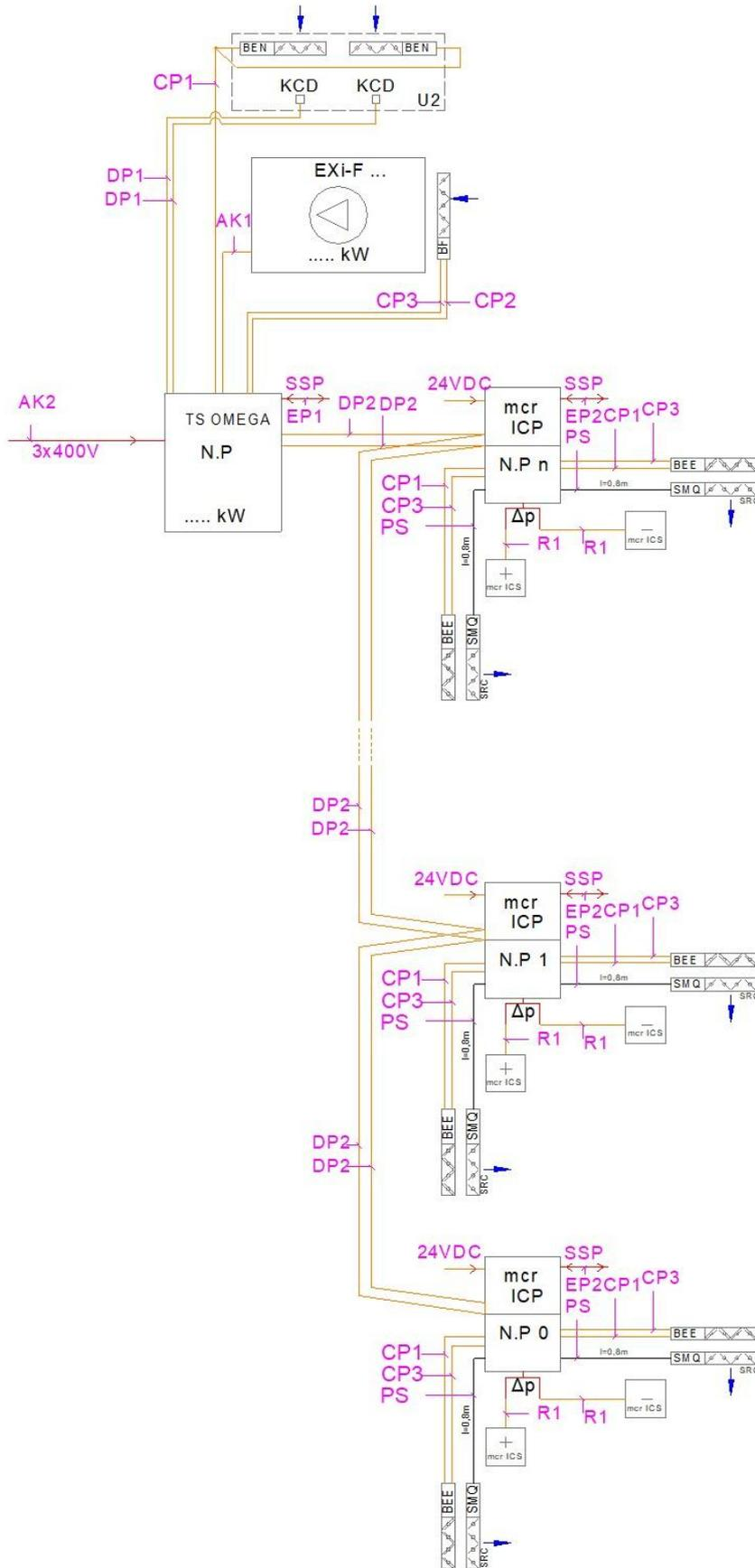
Figure 48 Schematic wiring diagram for a unit with high-speed mcr ICP dampers secured with smoke control system vents.
