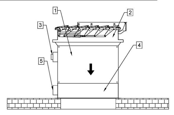
Figure 7 Sample installation of an air supply kit for the mcr EXi-F system in the UP version on the roof: 1 - fan, 2 - LAM vent with actuator, 3 - service disconnector or connection box, 4 - roof base, 5 - duct smoke detector.
