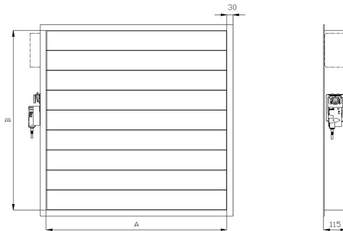
Figure 29 Overview of the EPSRC-B 9 damper (with additional connection box).
