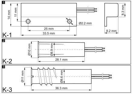
Figure 101 K-x series sensor installation dimensions.
