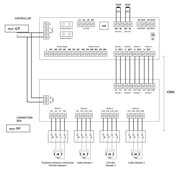
Figure 26 Connection of actuators to the mcr ICP regulator through the mcr PP connection box.
