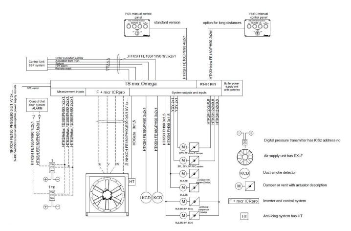
Figure 38 General electrical connection diagram for the EXi-F system: electrical connection, suggested types of wires for the mcr Omega control panel.
