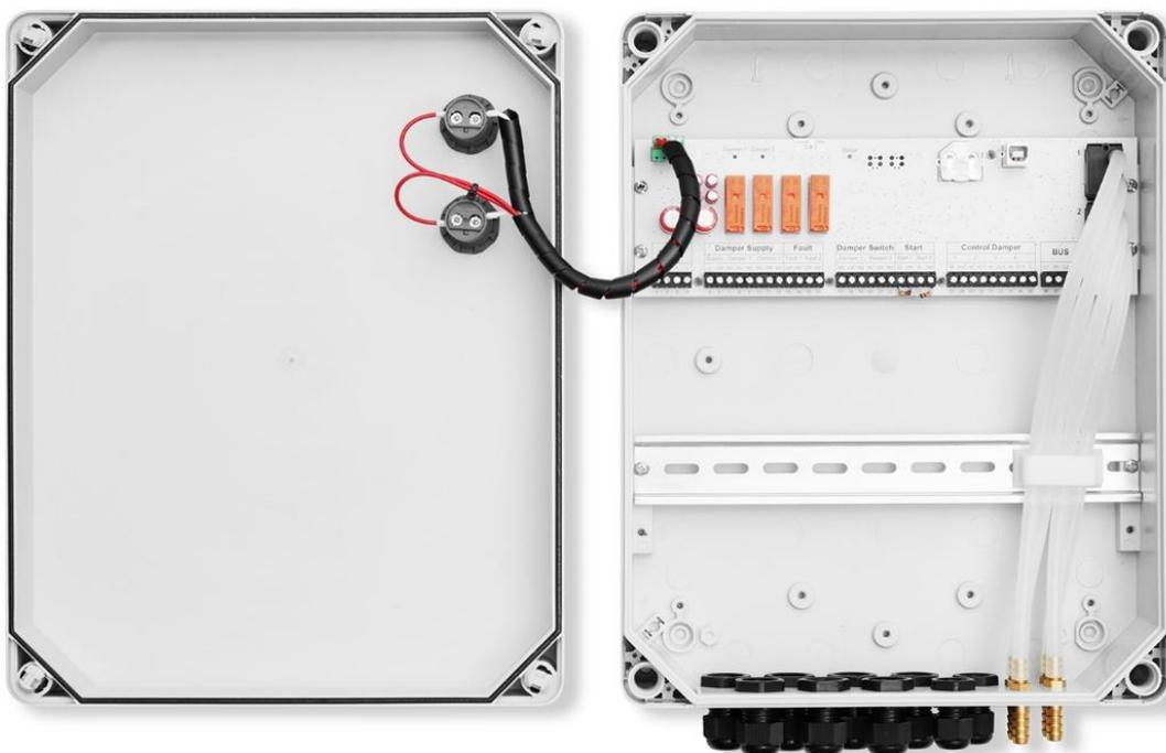
An example connection diagram is presented in Figure 31. Actuators are connected to the regulator only through a dedicated connection box. The box is equipped with a thermal fuse. The total length of cables between the regulator and the actuator must not exceed 15 m.
