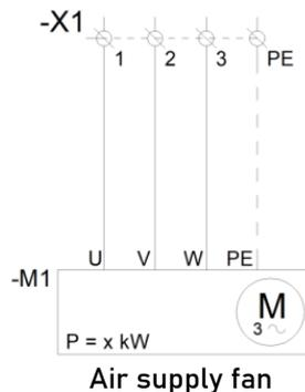
Figure 56 Fan connections circuit diagram.
