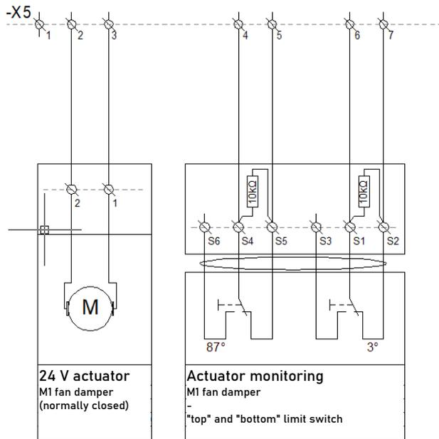
Figure 59 Shut-off damper actuator connections circuit diagram.
