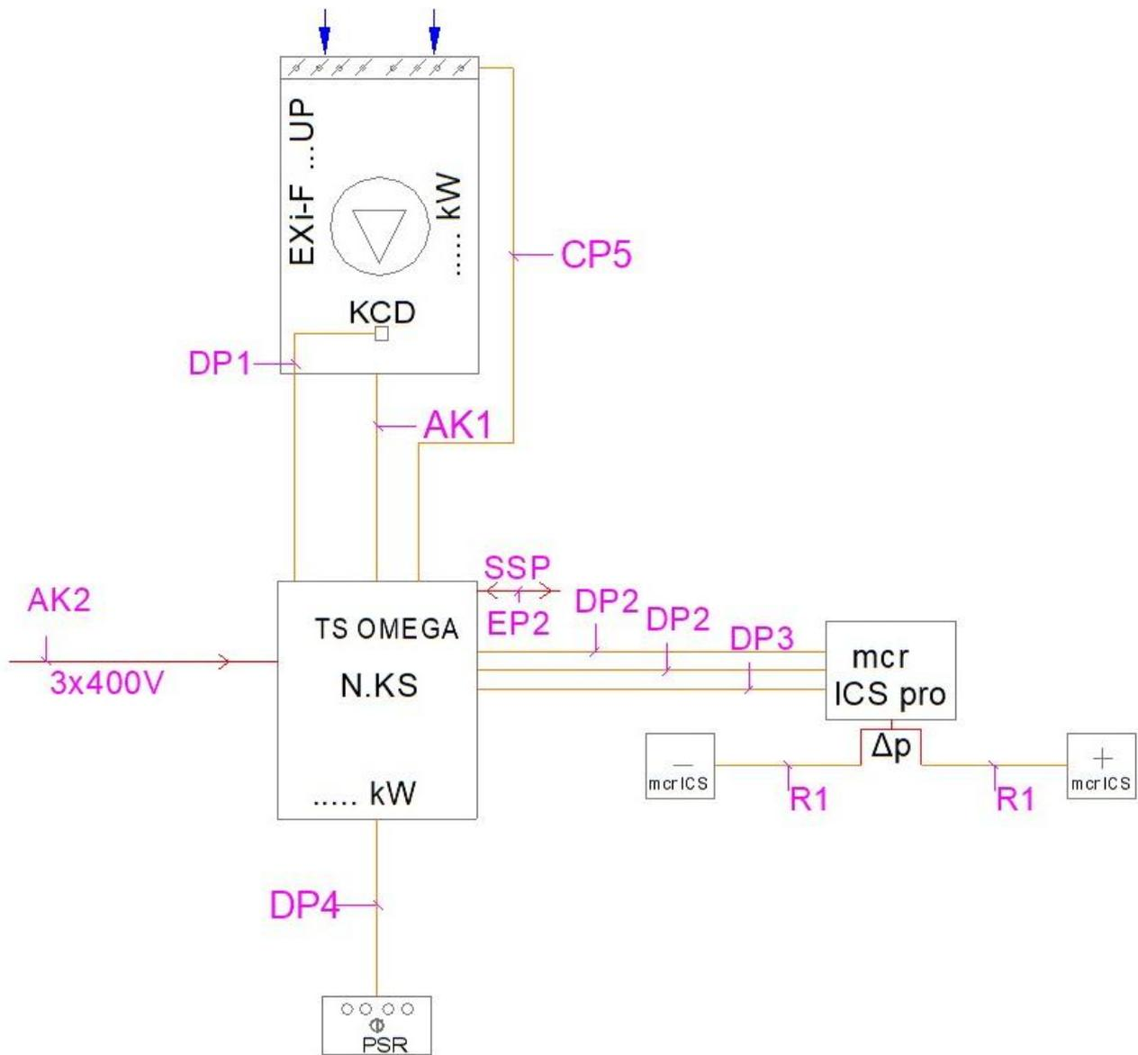
Figure 46 Schematic diagram of a vertical unit with a mcr LAM vent.
