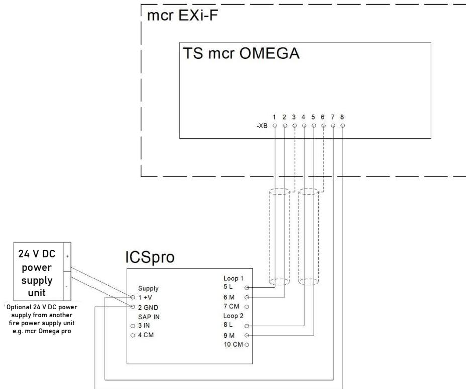
Figure 51 Block diagram for connecting a mcr ICS Pro pressure transmitter in a staircase-single transmitter setup.
