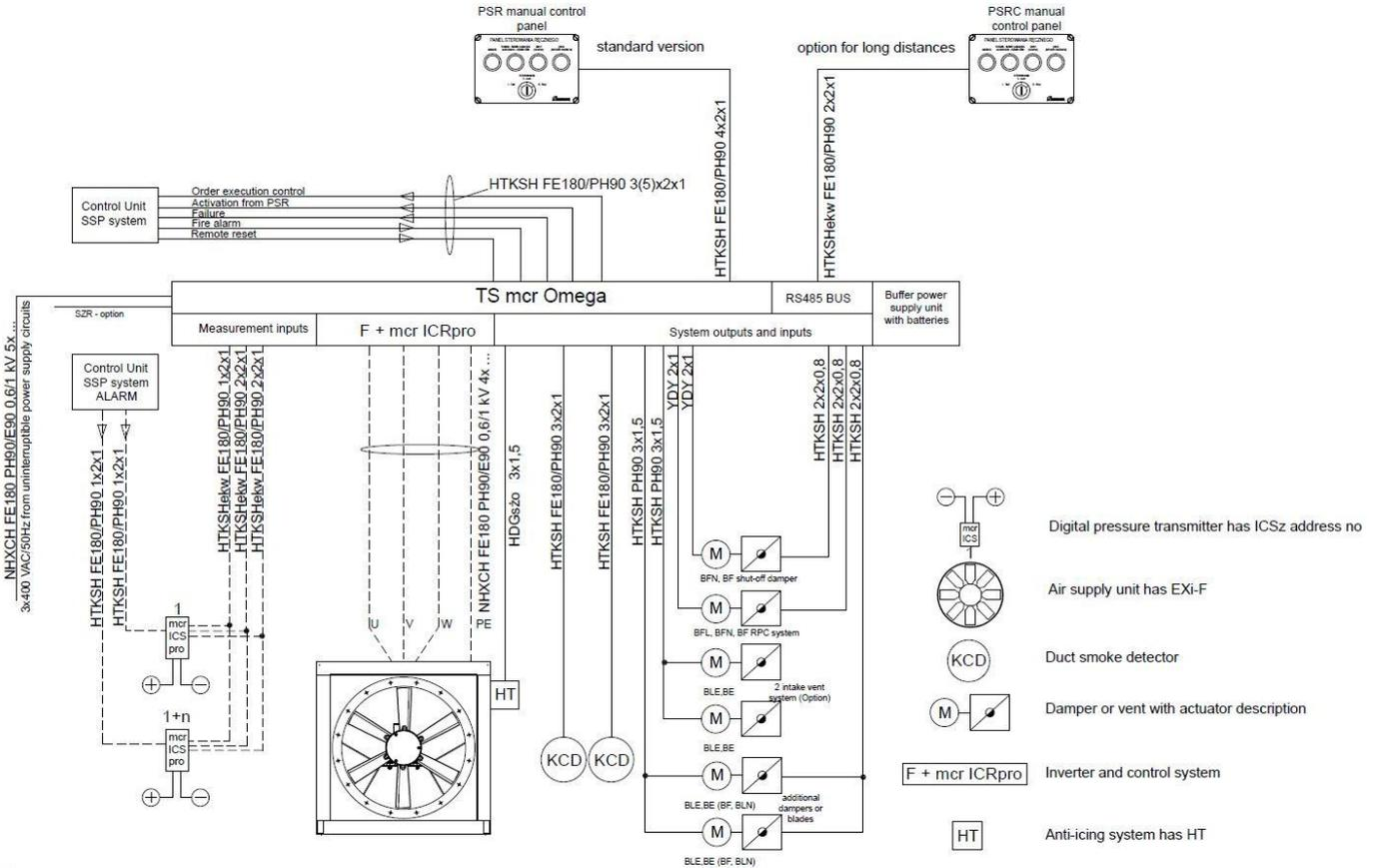
Figure 38 General electrical connection diagram for the EXi-F system: electrical connection, suggested types of wires for the mcr Omega control panel.
