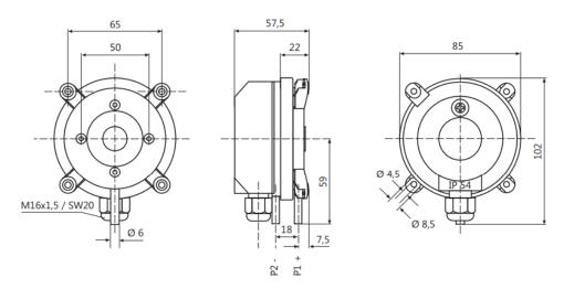
Figure 36 Differential pressure switch overview.
