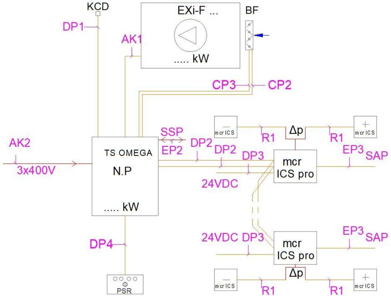
Figure 47 Schematic wiring diagram for lobby air supply.
