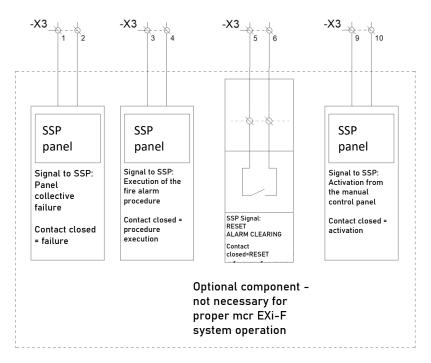
Figure 63 Connecting optional SSP signals to the mcr Omega panel.
