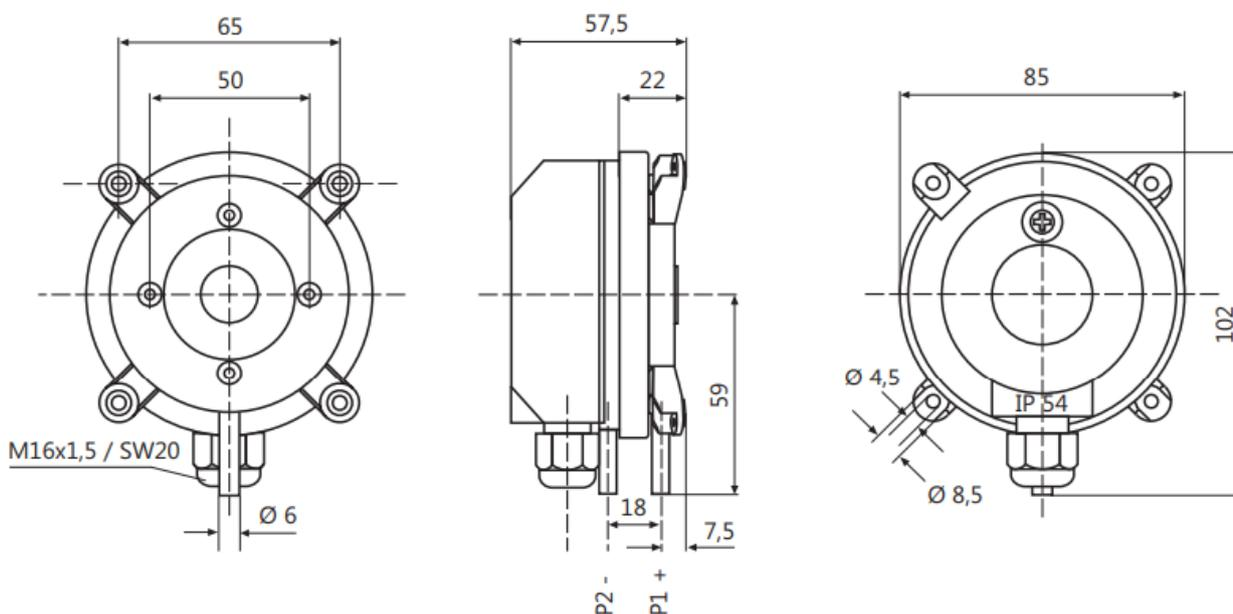
*Pressure input P1 (+) is connected downstream from the fan.
