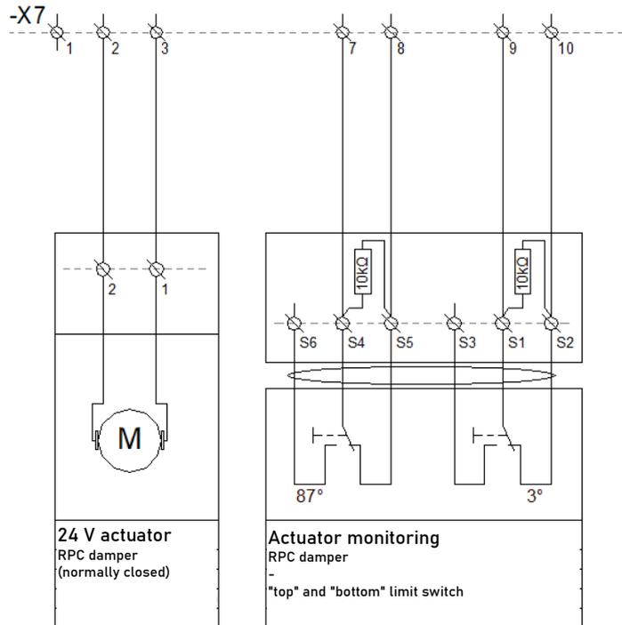
Figure 61 mcr RPC connections circuit diagram.
