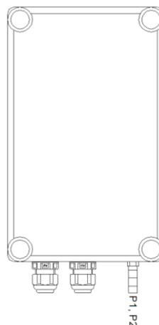
Figure 85 View of the mcr ICS pro differential pressure transmitter.
