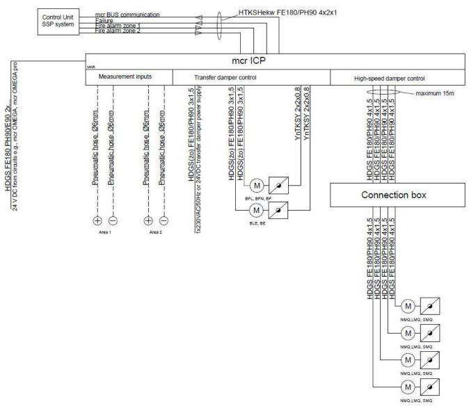
Figure 39 Electrical connection diagram for the mcr ICP lobby regulator handling 2 corridors and 4 high-speed dampers.
