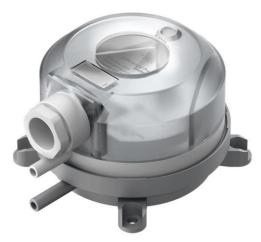
The differential pressure transmitters of the 984 series are used to measure differential pressure, overpressure and vacuum. For an optimum adaptation to the application, the transmitter can be switched between various pressure ranges. The factory setting is the most sensitive range. For the series 984M the less sensitive second range will be selected by simply removing a jumper. The output signal of the 3-wire version can be changed between 0-10 Volt and 4-20 mA by removing a jumper.
