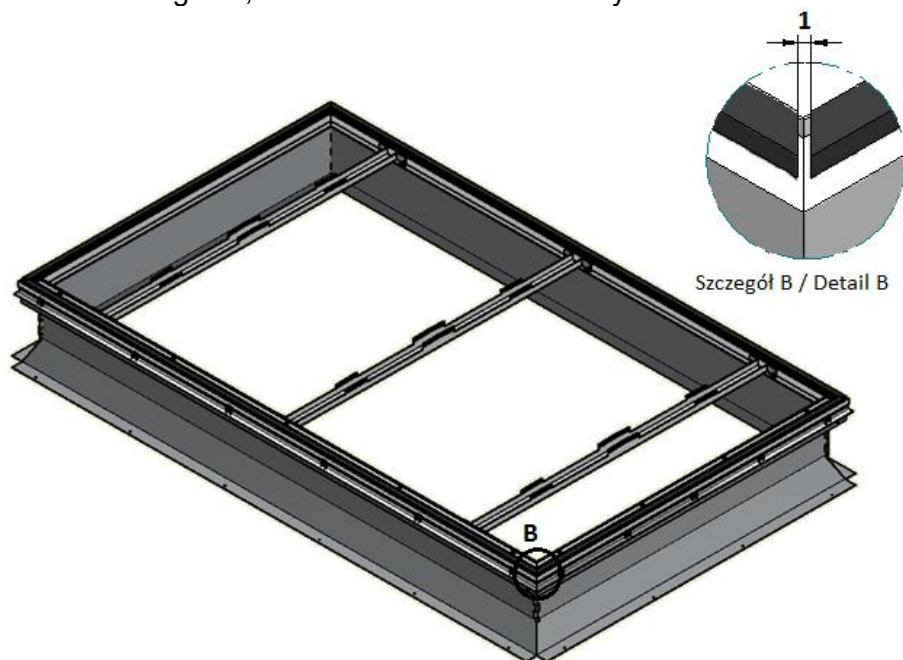
Fig. 45. Base of the FIX skylight with installed PVC top flange of base equipped with crossbeams and a PES 20x10 gasket
