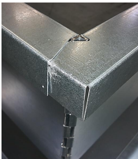
Fig. 25. Properly connected walls.
